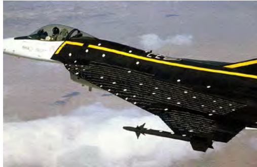
The F-16XL-1 was heavily instrumented for the CAWAP research program. The aircraft is seen during a data-collection run at an angle of attack of 21 degrees at an altitude of 17,500 feet. The surface tufts, pressure belts, and visual reference markings are readily discernible. (NASA)
