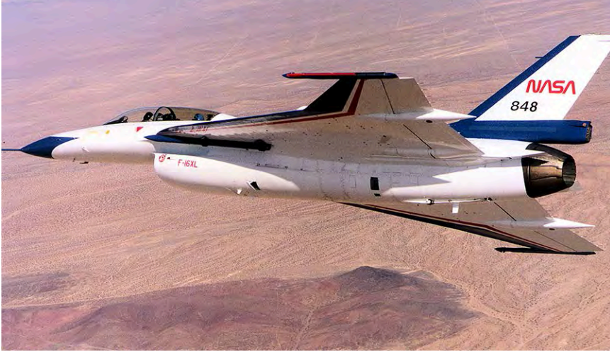
The two-seat F-16XL-2 powered by the F110-GE-129 engine seen on a test flight from NASA Dryden in October 1991. (NASA)
