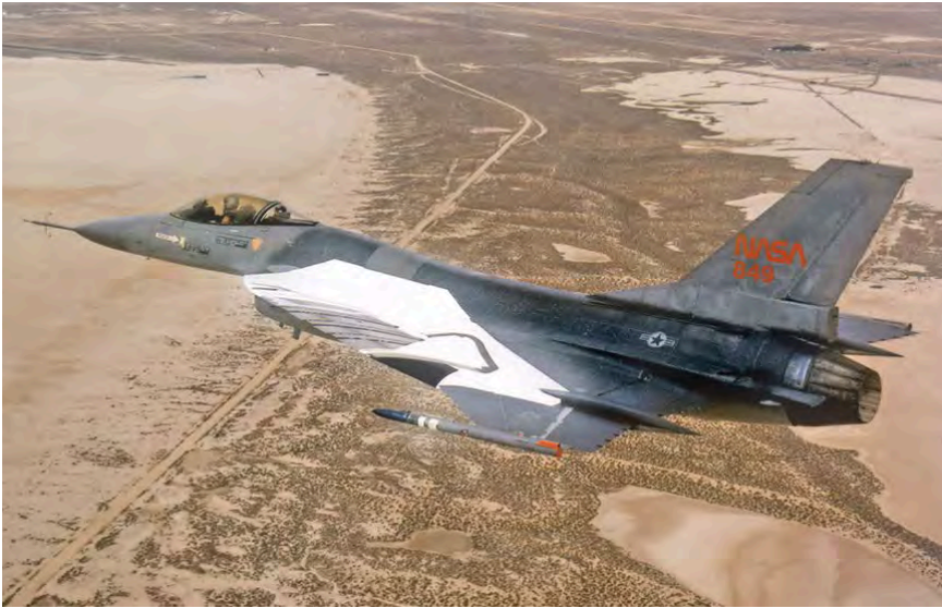
F-16XL-1 with the active suction glove on the left wing that was used for research into supersonic laminar flow control. The grey titanium active suction panel is visible on the inner region of the white wing glove. The passive outer leading edge of the wing glove is painted black in the region where a liquid-crystal sensor array was located. A video camera in the wingtip pod was used to record the liquid-crystal patterns. (NASA)
