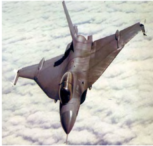
F-16XL-2 fitted with the extended air data boom used to measure angle of attack, yaw angle, and static and dynamic pressures. (USAF Photograph courtesy of SMSgt. Norman Taylor, USAF [ret.] )
