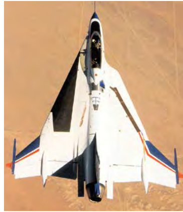
F-16XL-2 was fitted with wingtip-mounted DEI excitation vanes for flutter testing with the asymmetrical wing configuration that was used for NASA supersonic laminar flow research. (NASA)
