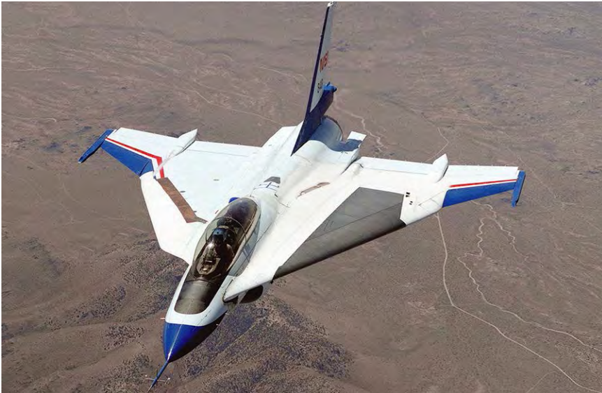
F-16XL-2 flying with a supersonic laminar flow control suction glove leading edge, April 1996. (NASA)
