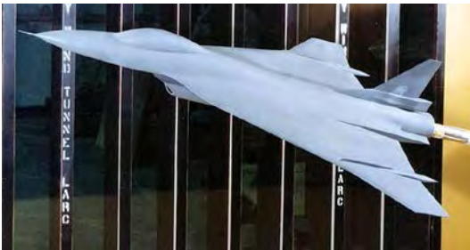
A near-final SCAMP–F-16XL configuration mounted in the LaRC Unitary Plan Wind Tunnel. The vertical tailfin was returned to the original F-16 production tail for improved lateral stability at higher angles of attack. (NASA)
