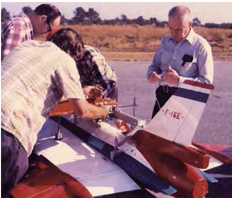
A radio-controlled 0.18-scale drop model is prepared for release from a NASA Bell HU-1 helicopter at the Plum Tree Island test facility in 1983. (NASA)
