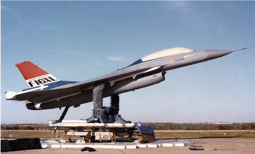
The F-16XL-2 during radar signature testing conducted by General Dynamics. (Lockheed Martin)
