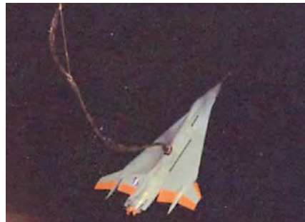
A free-flight model of the F-16XL with the wing apex modification seen during high-AoA free-flight testing in the Langley 30- by 60-foot wind tunnel. (NASA)
