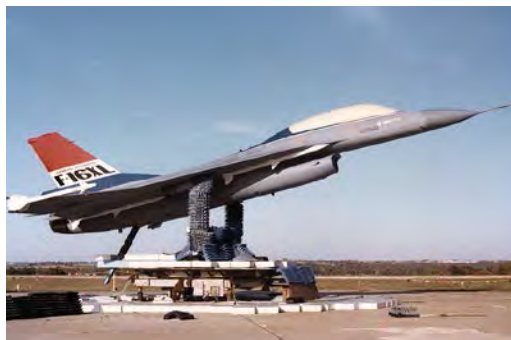
The F-16XL-2 during radar signature testing conducted by General Dynamics. (Lockheed Martin)
