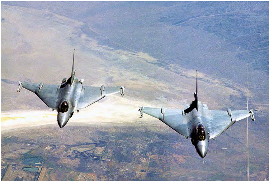
Both F-16XLs are seen in close formation with the full air-to-air missile payload of four AMRAAMs and two Sidewinders. The two-seat F-16XL-2 in the lead is painted in the so-called “Ferris” deceptive camouflage scheme. (USAF)
