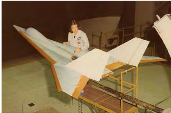
A wind tunnel force model of the NASA SCIF-4 supersonic cruise fighter configuration being prepared for testing at NASA Langley in 1977. (NASA)
