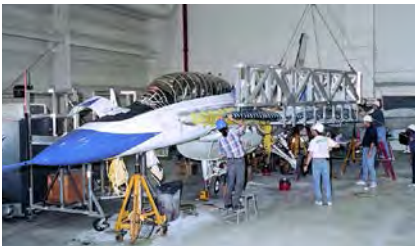
On left: The laminar flow wing glove during the positioning process on F-16XL-2's left wing, February 1995. On right: The F-16XL-2 after the laminar flow wing glove was mounted on the wing and the forward wing fairing was installed. Note how far forward on the fuselage the left wing extended. (Both images NASA)
