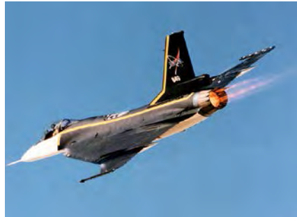
F-16XL-1 was used in its basic unmodified aerodynamic configuration for the CAWAP flight-test effort. (NASA)
