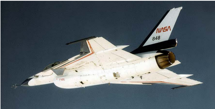
The F-16XL-2 in flight showing its Langley-tested shock wave fence under the port wing. (NASA)
