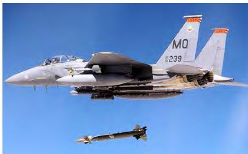
An F-15E Strike Eagle, of Air Combat Command's 391st Fighter Squadron, dropping a 5,000-pound GBU-28 deep-penetrating laser-guided bomb during exercises at the Utah Test and Training Range, August 2010. (USAF)
