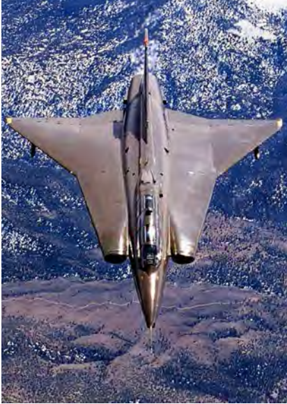
A two-place Saab Sk 35C Draken trainer of the National Test Pilot School cruising over the Sierra Nevada range on a training flight from Mojave Air and Space Port, Mojave, CA. Its "cranked-arrow" double-delta wing is readily apparent; the configuration anticipated by over a quarter century the cranked-arrow planform of the General Dynamics F-16XL. (National Test Pilot School photograph, courtesy Gregory V. Lewis and Russ Stewart)
