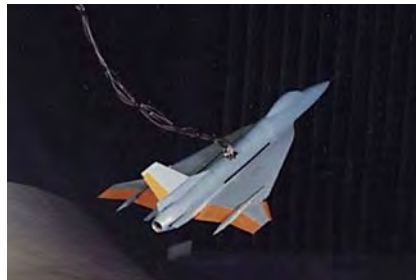
On left: NASA Langley's Sue Grafton is shown with the 0.18-scale captive free-flight wind tunnel model used to validate F-16XL aerodynamic and flight control modifications. On right: the 0.18-scale F-16XL model is seen during free-flight testing in the NASA Langley Full-Scale Tunnel. (Both images NASA)
