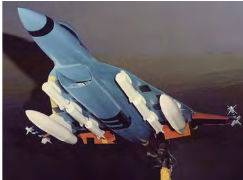
F-16XL wind tunnel test model fitted with six CBU-58 sub-munitions dispensers, two 370-gallon fuel tanks, and two wingtip-mounted AIM-9L missiles in the Langley Unitary Plan Wind Tunnel in 1982. (NASA)
