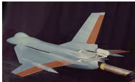
F-16XL model fitted with the "Quadra Pod" spin recovery parachute installation during wind tunnel testing at NASA Langley in May 1982. (NASA)
