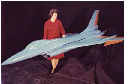
On left: NASA Langley's Sue Grafton is shown with the 0.18-scale captive free-flight wind tunnel model used to validate F-16XL aerodynamic and flight control modifications. On right: the 0.18-scale F-16XL model is seen during free-flight testing in the NASA Langley Full-Scale Tunnel. (Both images NASA)
