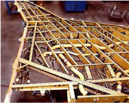
The robust internal structure of the F-16XL's cranked-arrow wing viewed looking outboard from the wing root toward the wingtip. (Lockheed Martin)
