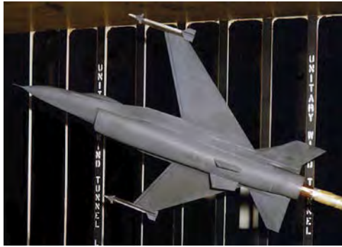
A wind tunnel test model of a modified F-16 fuselage fitted with a forward-swept wing mounted in the NASA Langley Unitary Plan Wind Tunnel in 1980. (NASA)
