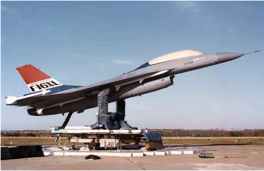
The F-16XL-2 during radar signature testing conducted by General Dynamics. (Lockheed Martin)
