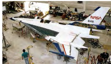
On left: The laminar flow wing glove during the positioning process on F-16XL-2's left wing, February 1995. On right: The F-16XL-2 after the laminar flow wing glove was mounted on the wing and the forward wing fairing was installed. Note how far forward on the fuselage the left wing extended. (Both images NASA)
