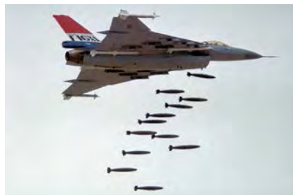
On left: The F-16XL-1 flying a test mission on August 18, 1982, with 12 500-pound Mk-82 bombs, 4 fuselage-mounted AIM-120 AMRAAMs, and 2 wingtip-mounted AIM-9 Sidewinder missiles. On right: On August 24, 1982, the F-16XL-1 successfully released 12 500 pound Mk-82 bombs from individual low-drag ejector bomb racks. (Both images USAF)
