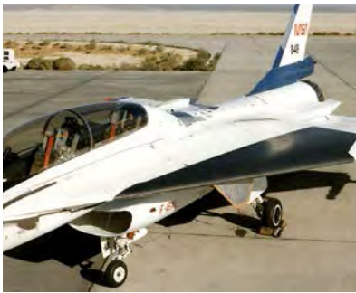
The F-16XL-2 seen with the 60-degree shock fence installed under the left inner wing in this November 1996 NASA Dryden photo. The fence was designed to block the shock waves that emanated from the engine inlet system. (NASA)
