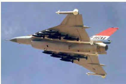
On left: The F-16XL-1 flying a test mission on August 18, 1982, with 12 500-pound Mk-82 bombs, 4 fuselage-mounted AIM-120 AMRAAMs, and 2 wingtip-mounted AIM-9 Sidewinder missiles. On right: On August 24, 1982, the F-16XL-1 successfully released 12 500 pound Mk-82 bombs from individual low-drag ejector bomb racks. (Both images USAF)
