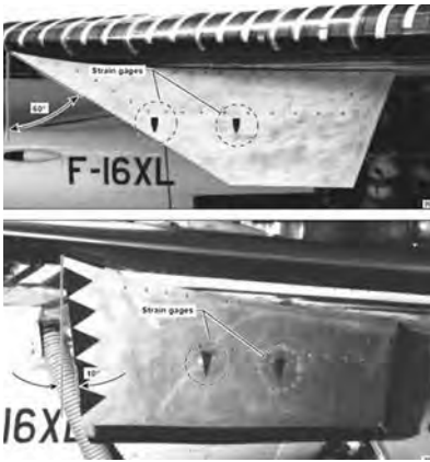
Different underwing shock wave fences were used to block the shock waves produced by the engine inlet from affecting the airflow on the leading edge of the wing glove. (NASA)
