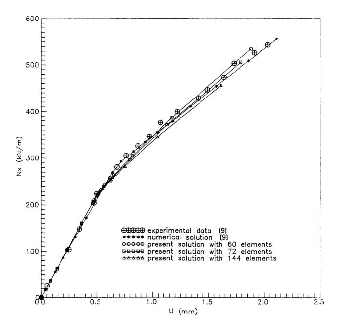
Fig. 2. Comparison among experimental data [9], current solutions (using 3-nodes triangular elements) and previous numerical results [9] for buckling and postbuckling response of a  $[\pm 45/0_2/\pm 45/0_2/\pm 45/0/90]_s$  composite under uniaxial compression
