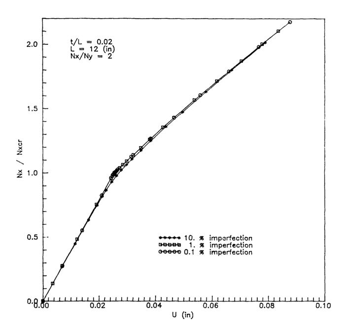
Fig. 10. Effect of imperfection sensitivity on buckling and postbuckling response of a clamped  $[0/90/\pm45]_{6s}$  plate under biaxial compression  $(N_x/N_y = 2, t/L = 0.02)$
