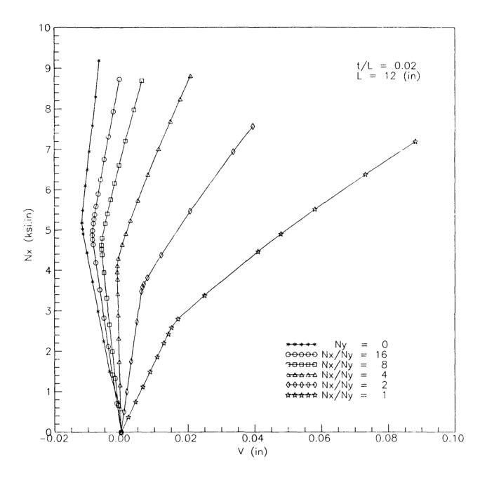
Fig. 22. Effect of stress-biaxiality ratio on buckling and postbuckling response (load  $N_X$  versus end-shortening V) along the Y-axis for a clamped  $[0/90/\pm45]_{6s}$  plate (t/L = 0.02)
