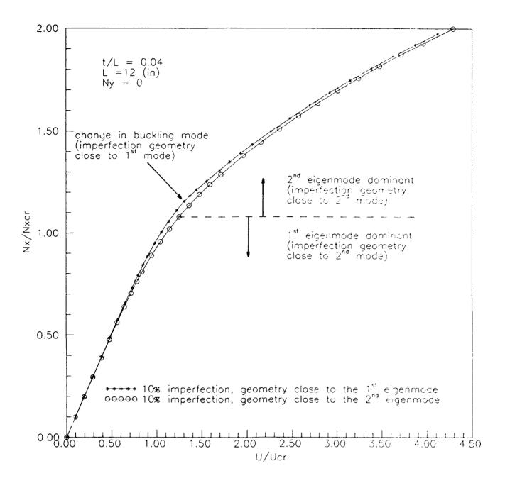
Fig. 18. Effect of imperfection geometry on buckling and postbuckling response (with a change in buckling mode) of a clamped  $[0/90/\pm45]_{12s} \ plate under uniaxial compression (10% imperfection, N_V = 0, t/L = 0.04)$
