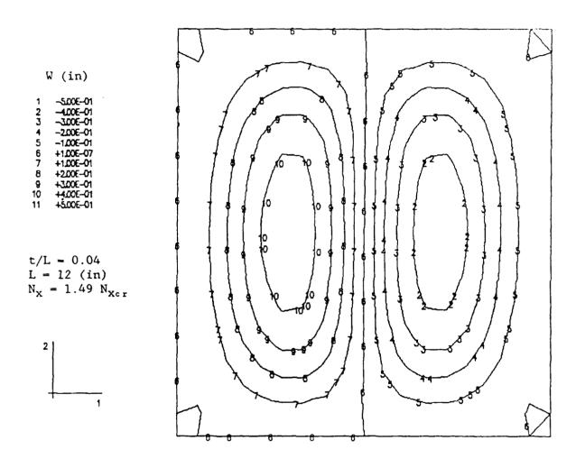
Fig. 12. Transverse displacements distribution after a change in buckling mode for a clamped  $[0/90/\pm45]_{12s}$  plate under uniaxial compression  $(N_X = 1.49 \ N_{Xcr}, 1\% \ imperfection, t/L = 0.04)$
