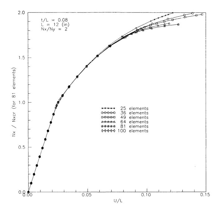
Fig. 5. Effect of mesh refinement on buckling and postbuckling solution convergence for a clamped  $[0/90/\pm45]_{24s}$  plate under biaxial compression  $(N_x/N_y = 2, t/L = 0.08)$
