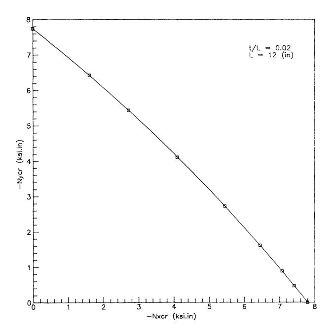
Fig. 20. Critical load-stability envelope for a clamped  $[0/90/\pm45]_{6s}$  plate under biaxial states of stress (t/L = 0.02)
