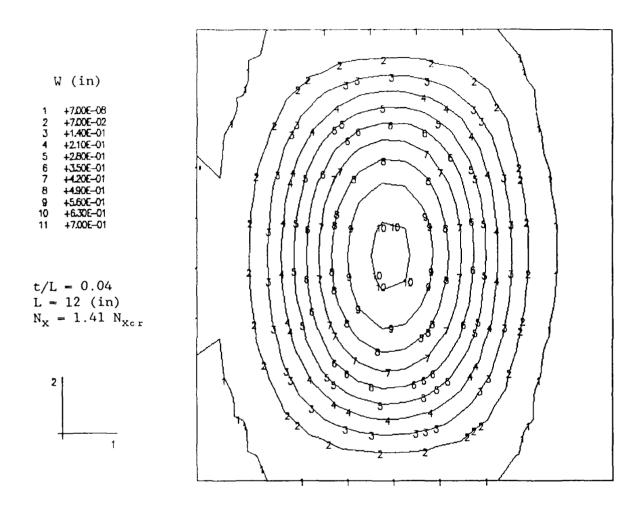
Fig. 11. Transverse displacements distribution before a change in buckling mode for a clamped  $[0/90/\pm45]_{12s}$  plate under uniaxial compression  $(N_x = 1.41 N_{xcr}, 1% imperfection, t/L = 0.04)$
