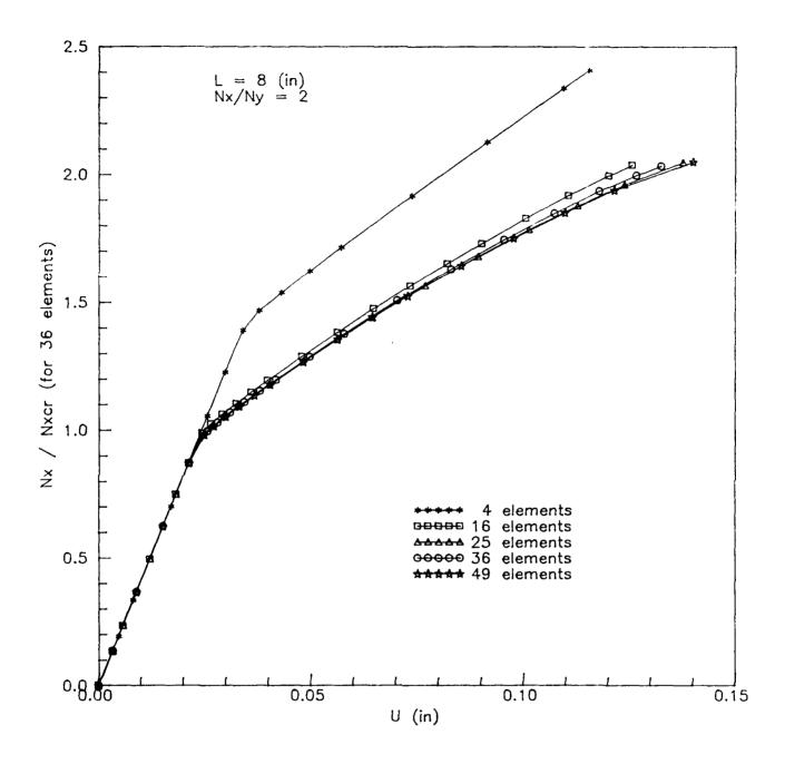
Fig. 4. Effect of mesh refinement on buckling and postbuckling solution convergence for a clamped unidirectional plate under biaxial compression  $(N_x/N_y = 2, t/L = 0.05)$
