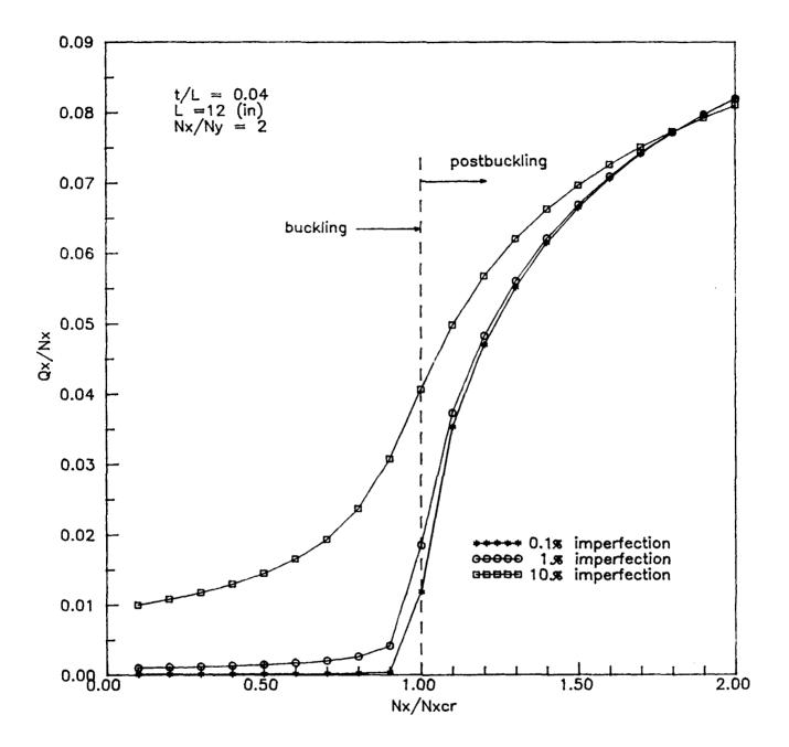
Fig. 26. Effect of imperfection sensitivity on transverse shear  $Q_x$  at (-3,-3) (in) in a clamped  $[0/90/\pm45]_{12s}$  plate under biaxial compression  $(N_x/N_y=2,\ t/L=0.04)$
