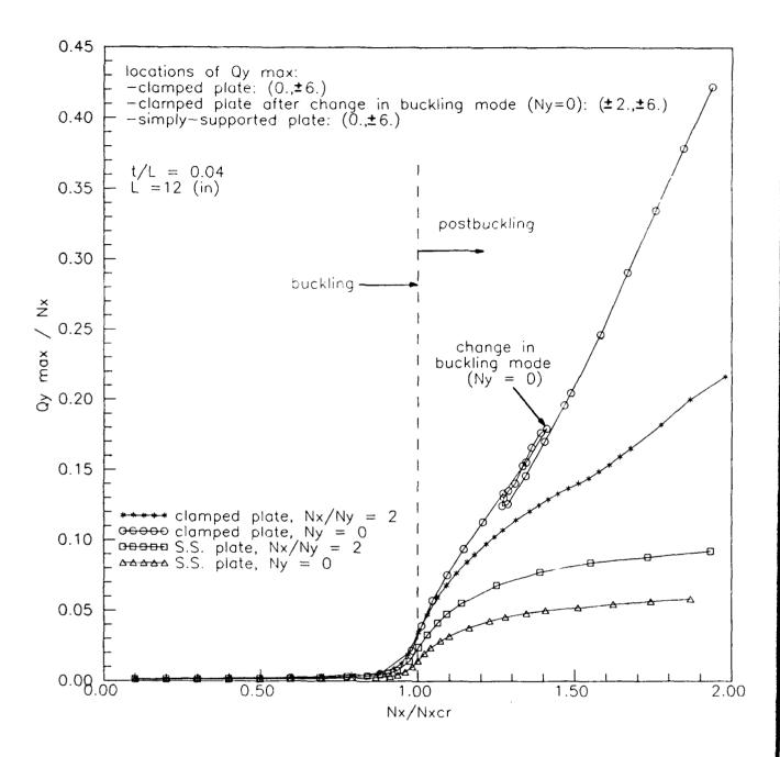
Fig. 29. Effects of boundary conditions and stress-biaxiality on maximum transverse shear  $Q_y$  in a  $[0/90/\pm45]_{12s}$  laminate (t/L = 0.04)
