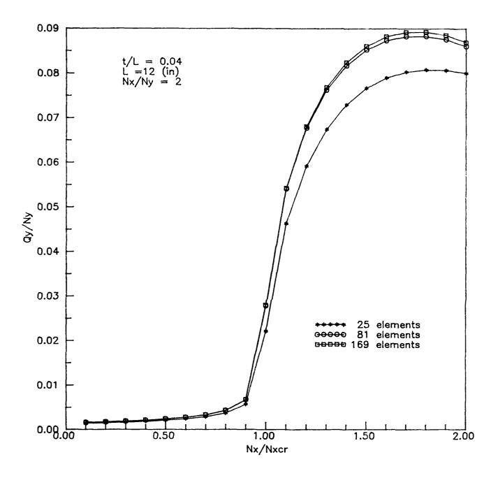
Fig. 8. Solution convergence for transverse shear  $Q_y$  at (-3,-3) (in) in a clamped  $[0/90/\pm45]_{12s}$  plate under biaxial compression  $(N_x/N_y=2,\ t/L=0.04)$
