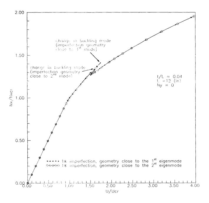
Fig. 19. Effect of imperfection geometry on buckling and postbuckling response (with a change in buckling mode) of a clamped  $[0/90/\pm45]_{12s} \text{ plate under uniaxial compression (1% imperfection.} \\ N_{\gamma} = 0, \ t/L = 0.04)$
