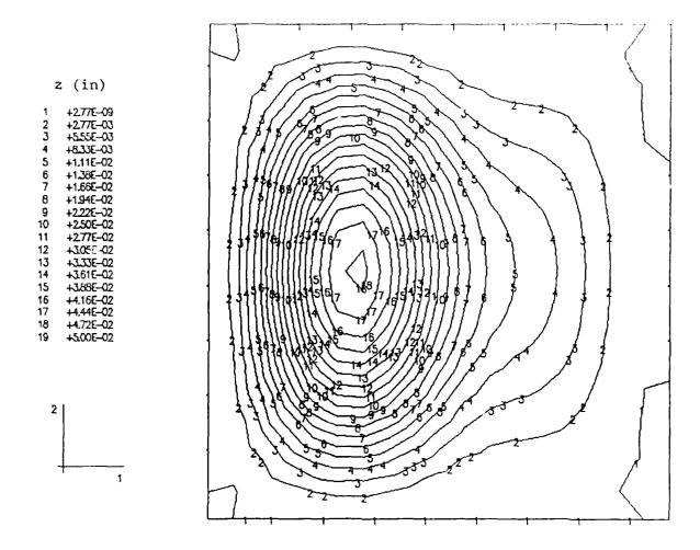
Fig. 16. Constructed imperfection geometry close to the first eigenmode for a 10% imperfection
