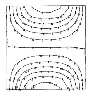
Fig. 31. Distribution of transverse shear  $Q_y$  at  $N_x = 1.5 \ N_{xcr}$  in a simply-supported  $[0/90/\pm45]_{12s}$  plate under biaxial compression  $(N_x/N_y = 2, \ t/L = 0.04)$
