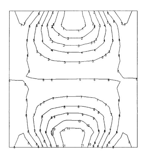
Fig. 33. Distribution of transverse shear  $Q_y$  at  $N_x = 1.5 \ N_{xcr}$  in a clamped  $[0/90/\pm45]_{12s}$  plate under biaxial compression  $(N_x/N_y = 2, \ t/L = 0.04)$
