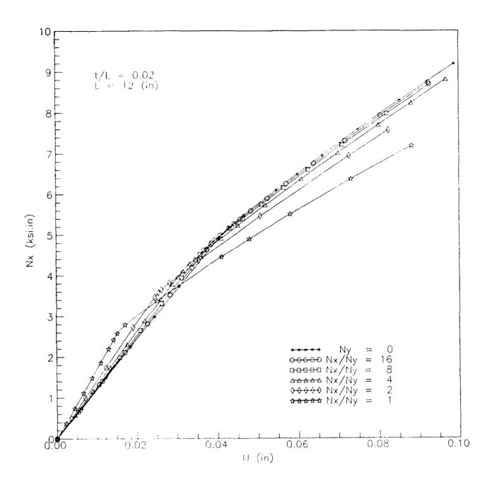
Fig. 21. Effect of stress-biaxiality ratio on buckling and postbuckling response (load  $N_X$  versus end-shortening U) along the X-axis for a clamped  $[0/90/\pm45]_{6s}$  plate (t/L = 0.02)
