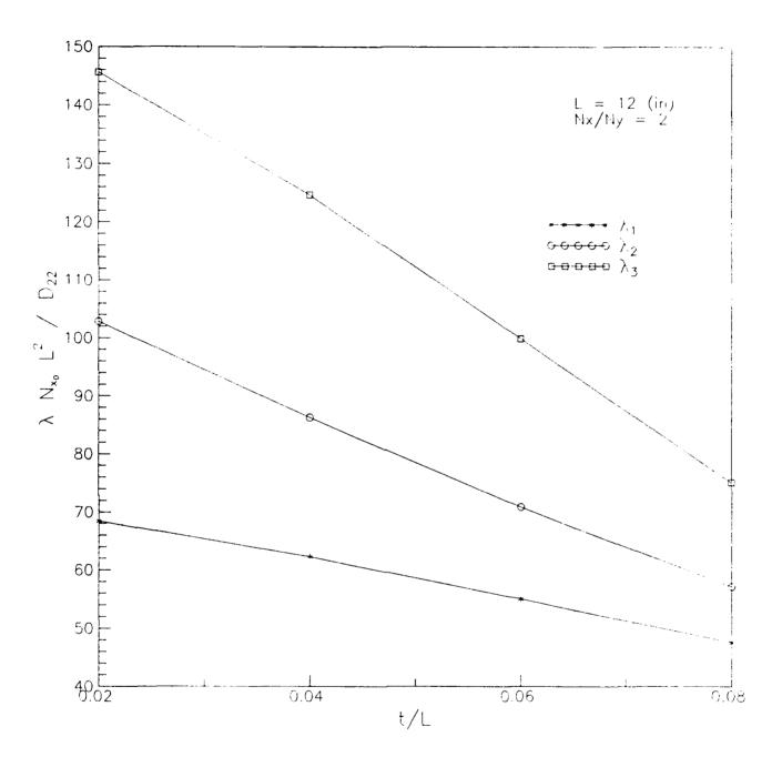
Fig. 35. Effect of laminate thickness on lowest three eigenvalues of a clamped  $[0/90/\pm45]_{ns}$  plate under biaxial compression  $(N_X/N_y-2)$
