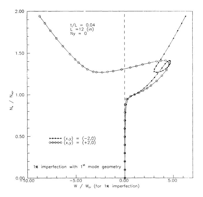
Fig. 14. Transverse displacements W at  $(\pm 2.0)$  for a clamped  $[0/90/\pm 45]_{12s}$  plate under uniaxial compression (1% imperfection, N<sub>y</sub> = 0, t/L = 0.04)
