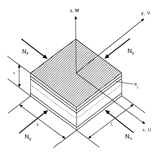
Fig. 1. Coordinates and geometry of a composite laminate plate under compressive loading
