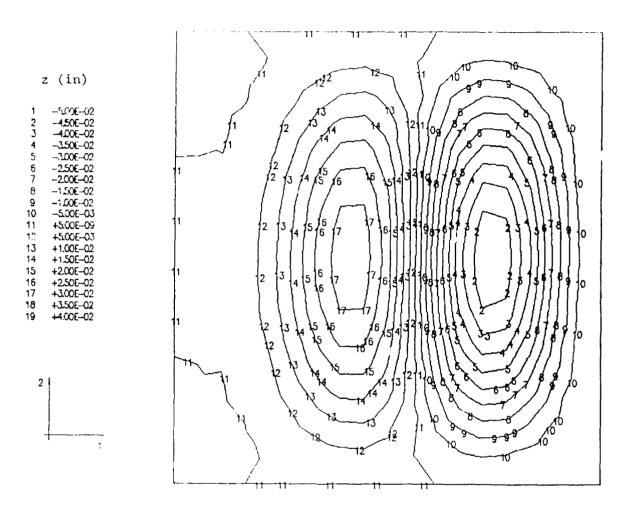
Fig. 17. Constructed imperfection geometry close to the second eigenmode for a 10% imperfection
