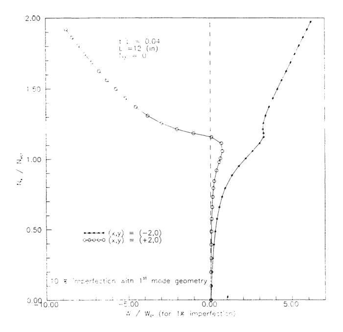
Fig. 15. Transverse displacements W at  $(\pm 2.0)$  for a clamped  $[0/90/\pm 45]_{12s}$  plate under uniaxial compression (10% imperfection,  $N_y = 0$ , t/L = 0.04)
