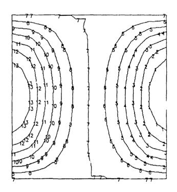
Fig. 30. Distribution of transverse shear  $Q_X$  at  $N_X$  = 1.5  $N_{Xcr}$  in a simply-supported  $[0/90/\pm45]_{12s}$  plate under biaxial compression  $(N_x/N_y = 2, t/L = 0.04)$
