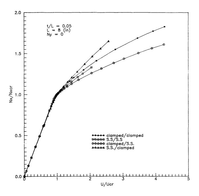
Fig. 23. Effect of boundary conditions on buckling and postbuckling response of a unidirectional laminate plate under uniaxial compression  $(N_{\psi}=0,\ t/L=0.05)$
