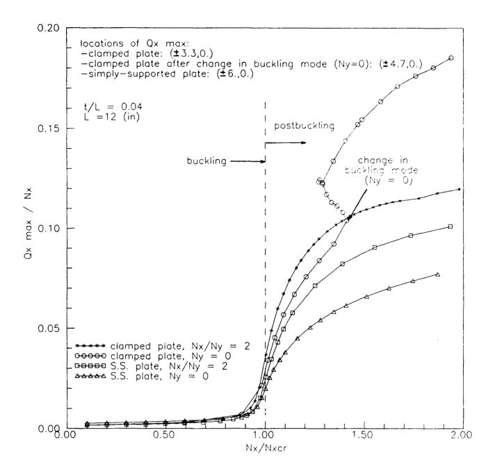
Fig. 28. Effects of boundary conditions and stress-biaxiality on maximum transverse shear  $Q_X$  in a  $[0/90/\pm45]_{12s}$  laminate (t/L=0.04)
