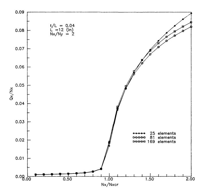
Fig. 7. Solution convergence for transverse shear  $Q_X$  at (-3,-3) (in) in a clamped  $[0/90/\pm45]_{12s}$  plate under biaxial compression  $(N_X/N_y=2,\ t/L=0.04)$
