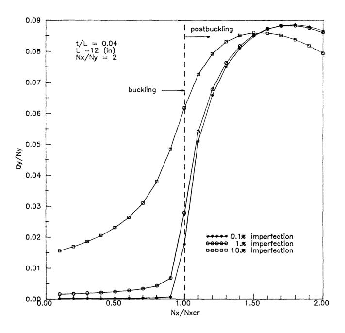
Fig. 27. Effect of imperfection sensitivity on transverse shear  $Q_y$  at (-3,-3) (in) in a clamped  $[0/90/\pm45]_{12s}$  plate under biaxial compression  $(N_x/N_y=2,\ t/L=0.04)$
