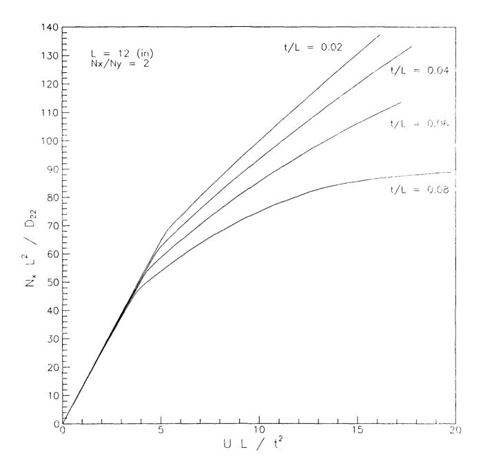
Fig. 34. Effect of laminate thickness on buckling and postbuckling response of a clamped  $[0/90/\pm45]_{ns}$  plate under biaxial compression  $(N_x/N_y=2)$
