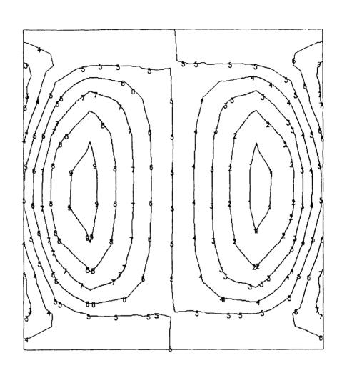
Fig. 32. Distribution of transverse shear  $Q_X$  at  $N_X = 1.5~N_{Xcr}$  in a clamped  $[0/90/\pm45]_{12s}$  plate under biaxial compression  $(N_X/N_y = 2,~t/L = 0.04)$
