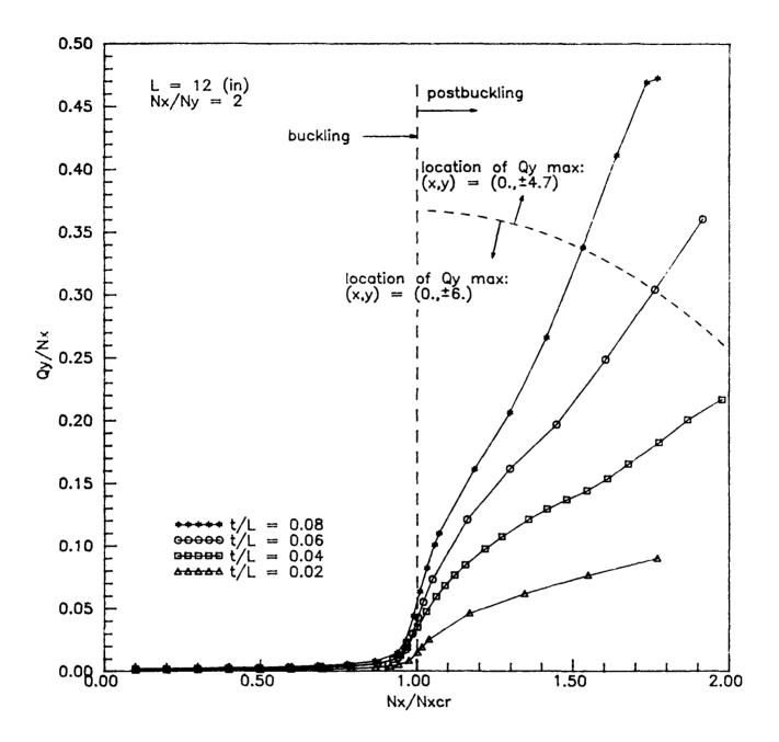
Fig. 37. Effect of laminate thickness on maximum transverse shear  $Q_y$  in buckling and postbuckling response of a clamped  $[0/90/\pm45]_{\rm ns}$  plate under biaxial compression  $(N_{\rm X}/N_{\rm y}=2)$
