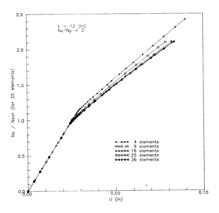
Fig. 3. Effect of mesh refinement on buckling and postbuckling solution convergence for a clamped  $[0/90/\pm45]_{6s}$  plate under biaxial compression  $(N_x/N_y=2,\ t/L=0.02)$
