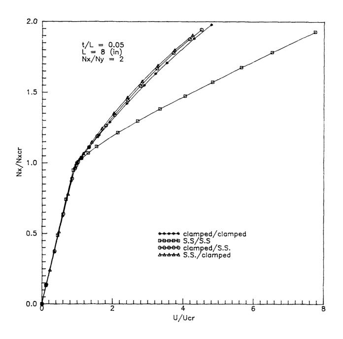
Fig. 24. Effect of boundary conditions on buckling and postbuckling response of a unidirectional laminate plate under biaxial compression  $(N_{\rm X}/N_{\rm Y}=2,\ t/L=0.05)$
