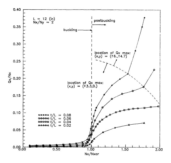
Fig. 36. Effect of laminate thickness on maximum transverse shear  $Q_X$  in buckling and postbuckling response of a clamped  $[0/90/\pm45]_{\rm BS}$  plate under biaxial compression  $(N_X/N_Y=2)$
