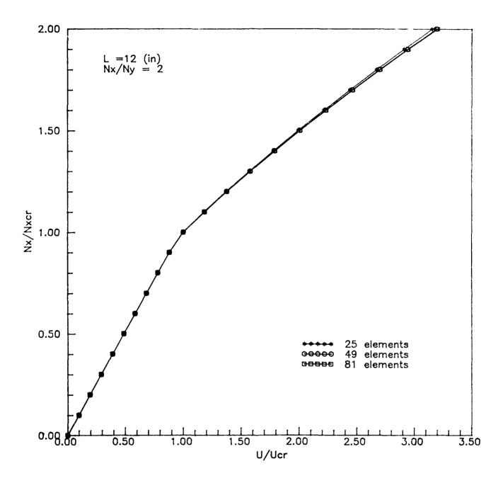
Fig. 6. Effect of mesh refinement on buckling and postbuckling solution convergence for a clamped  $[0/90/\pm45]_{12s}$  plate under biaxial compression  $(N_x/N_y=2,\ t/L=0.04)$
