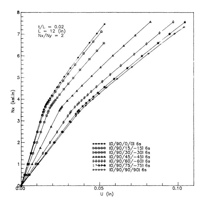
Fig. 25. Effect of lamination layup on buckling and postbuckling response of clamped plates under biaxial compression ( $N_x/N_y$  = 2, t/L = 0.02)
