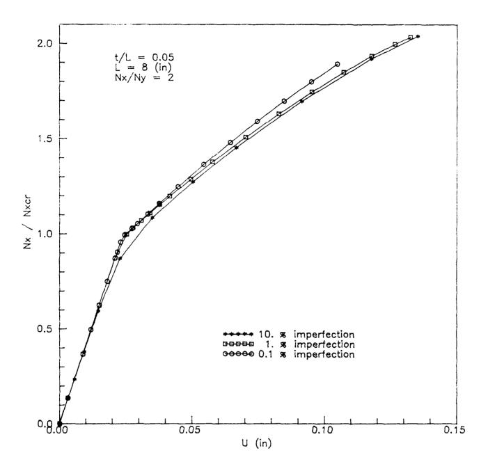
Fig. 9. Effect of imperfection sensitivity on buckling and postbuckling response of a clamped unidirectional composite plate under biaxial compression  $(N_X/N_y=2,\ t/L=0.05)$
