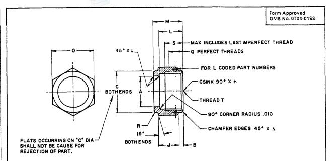
(a) DIMENSION A AND THREAD T SHALL BE CONCENTRIC WITHIN .005 FIM.
