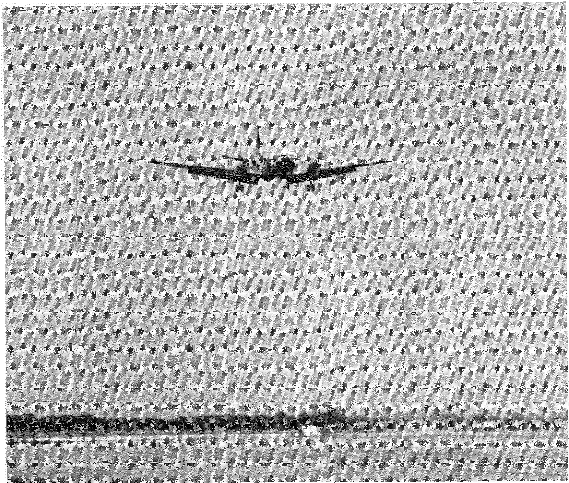
Fig 5. Andover approaching over vertical water jet barrier
