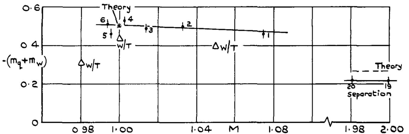
Fig.18 Damping-in-pitching derivative  $m_q + m_w$
