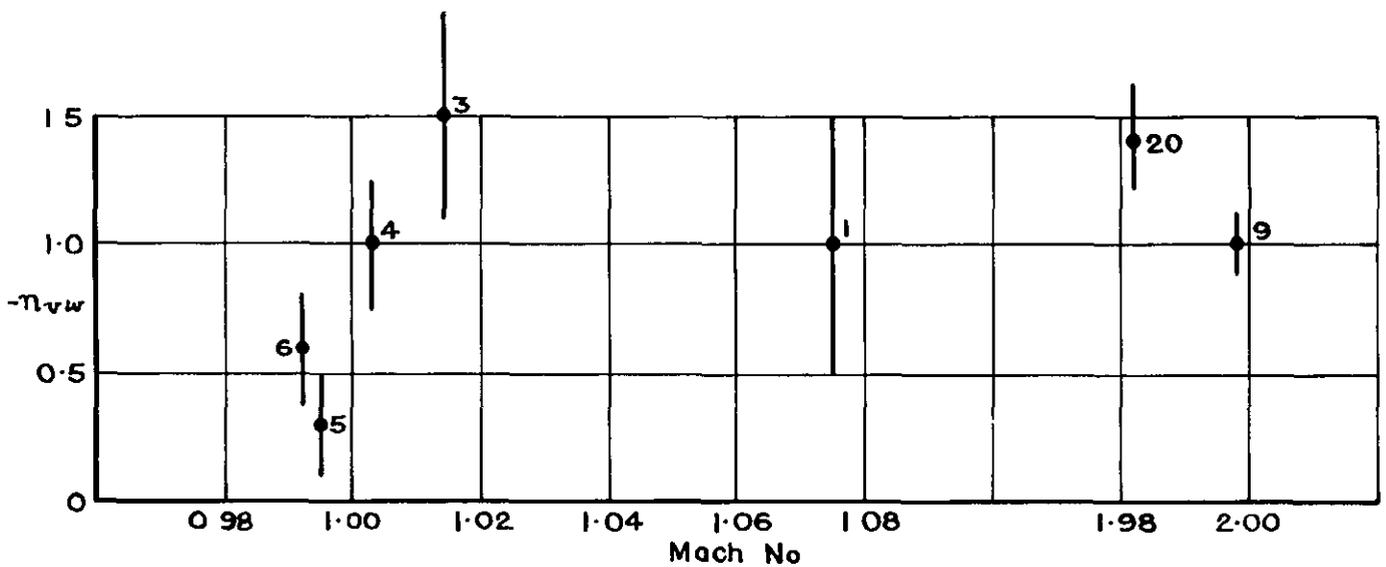
Fig.29 Yawing moment due to combined sideslip and incidence,  $n_{vw}$
