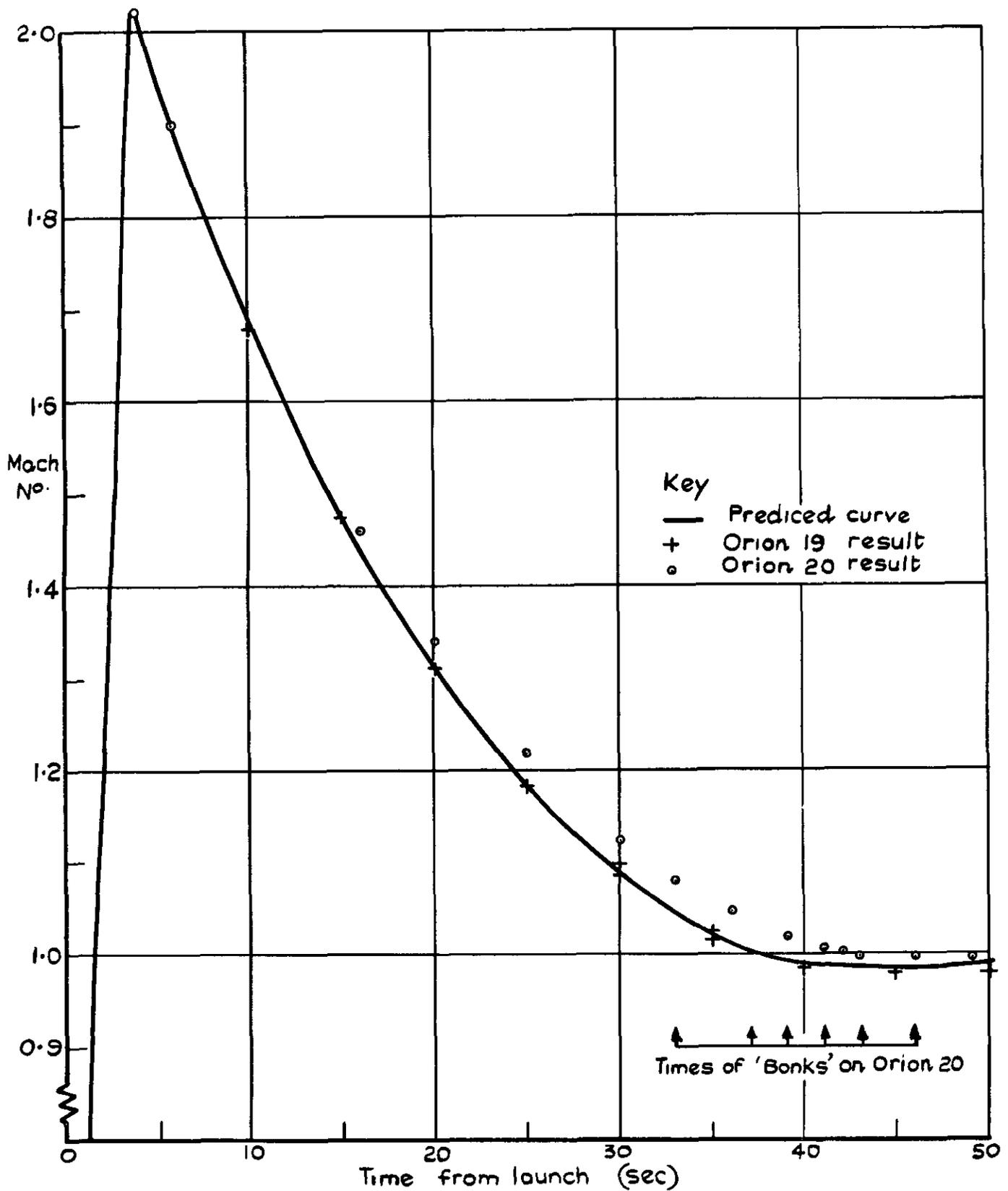
Fig.6 Comparison of the predicted variation of Mach N<sup>o</sup>. with time, with the actual results from Orions 19 and 20.
