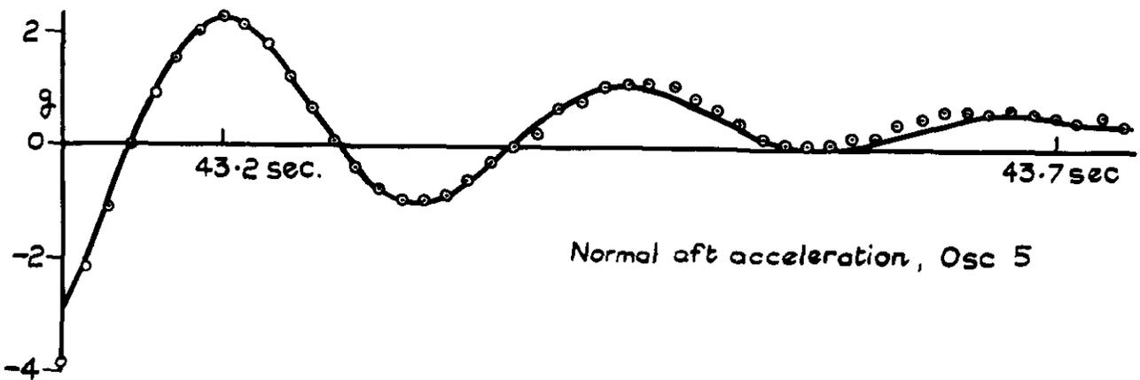
Fig.15 Some examples of best fit to normal aft acceleration on Orion 20
