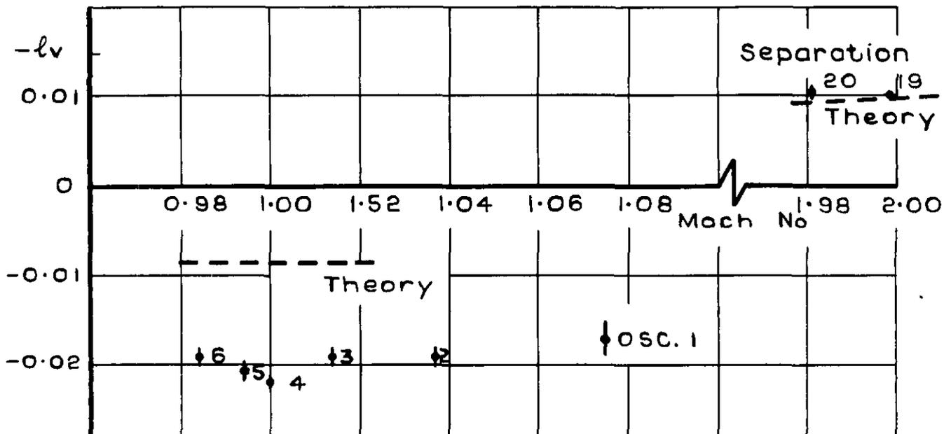
Fig 20 Rolling moment due to sideslip,  $l_v$
