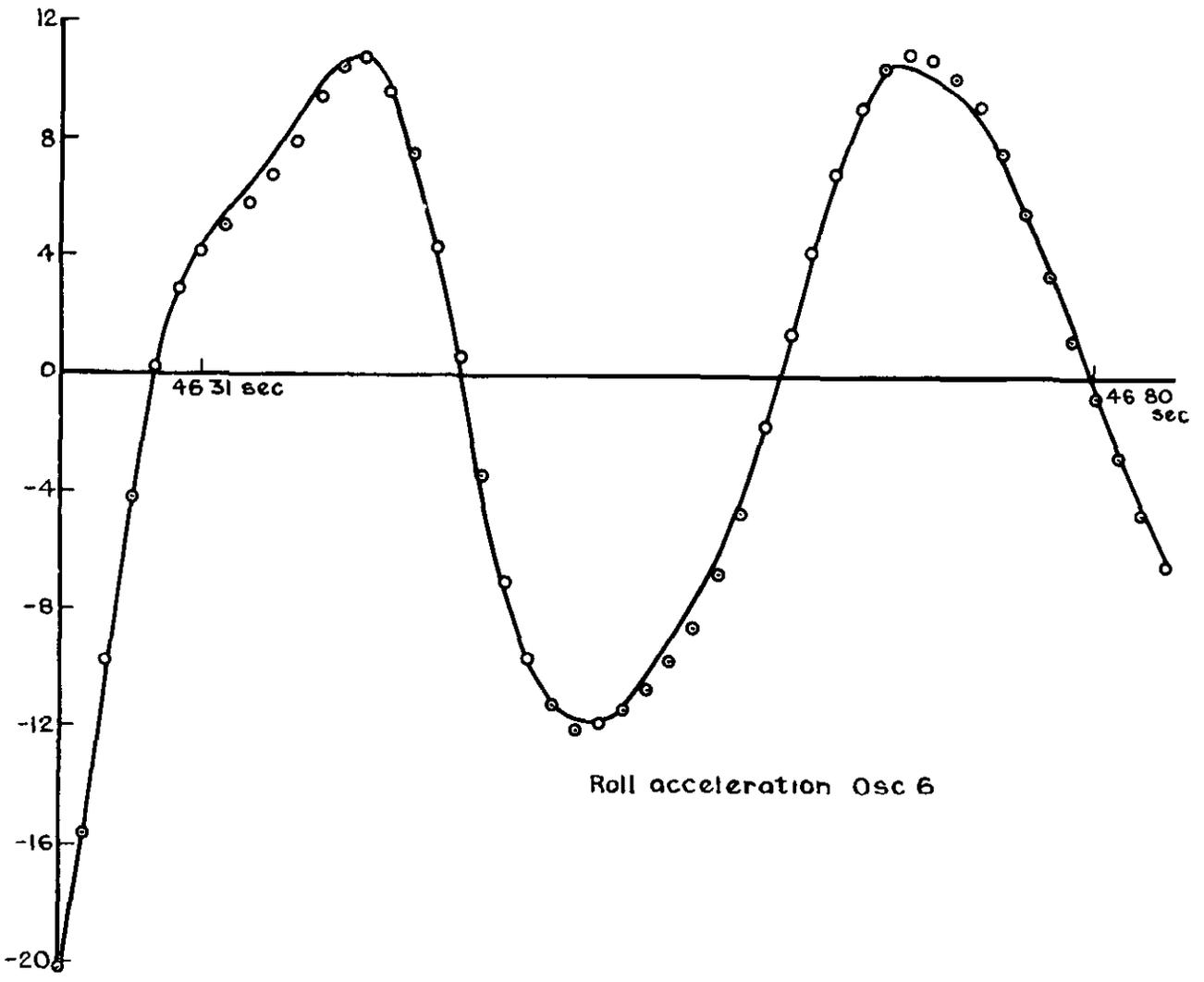
Fig.19 Some examples of best fit to roll acceleration on Orion 20
