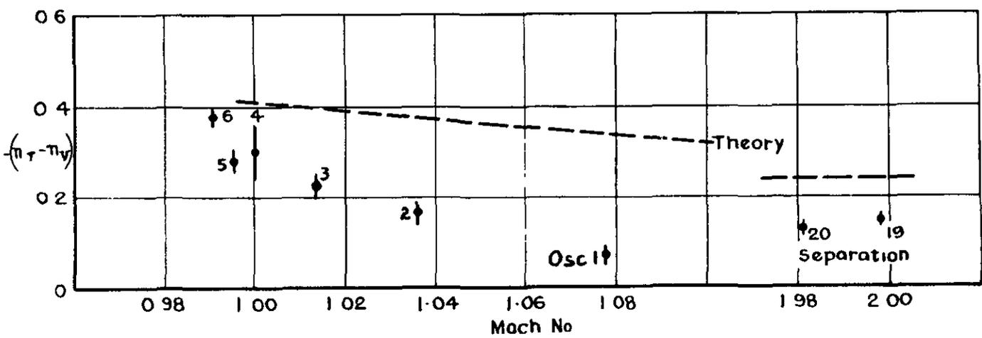
Fig.26 Damping-in-yaw derivative,  $n_r - n_v$
