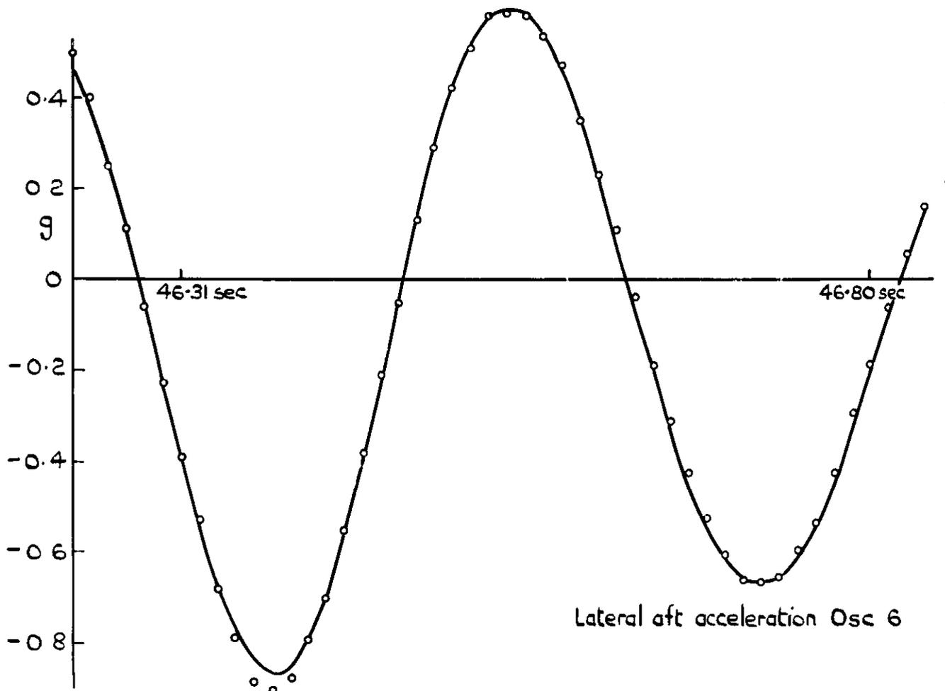
Fig. 23 Some examples of best fit to lateral acceleration on Orion 20
