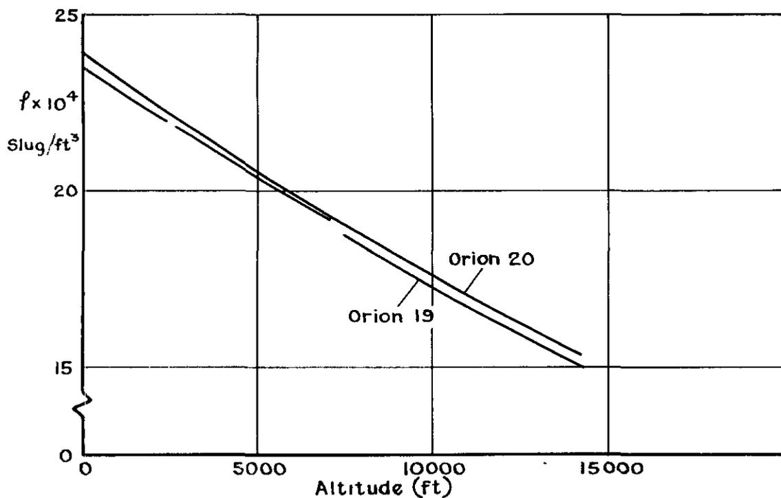
Fig. 8 Measured air density compared with standard atmosphere
