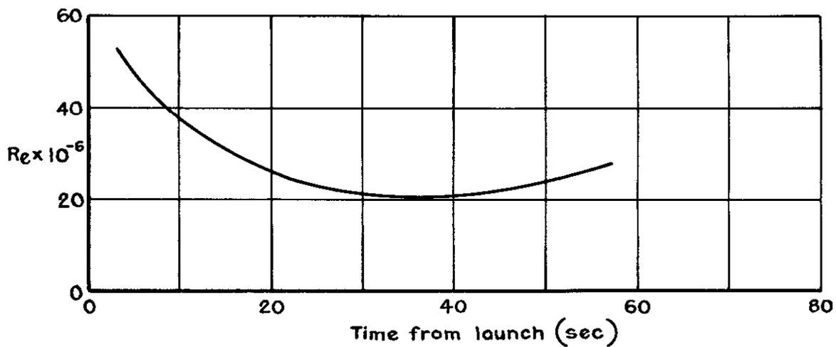
Fig.11 Reynolds number (based on  $\bar{C}$ ) for Orion 20
