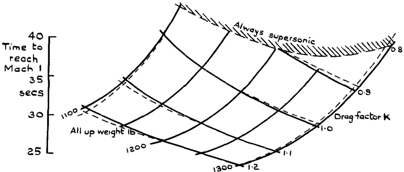
Fig.3 Time to reach Mach No 1 as a function of model drag factor and all-up weight of Orion on solid fuel boost
