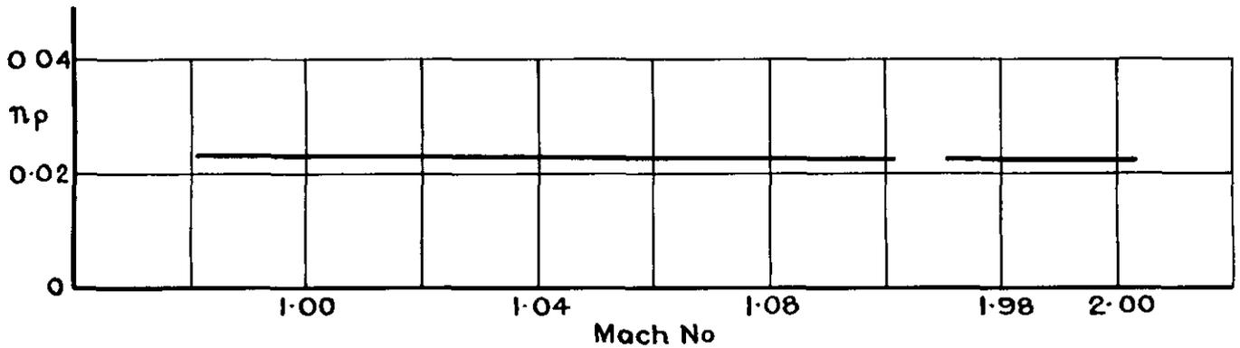
Fig.28 Theoretical yawing moment due to rate of roll,  $n_p$  assumed for analysis
