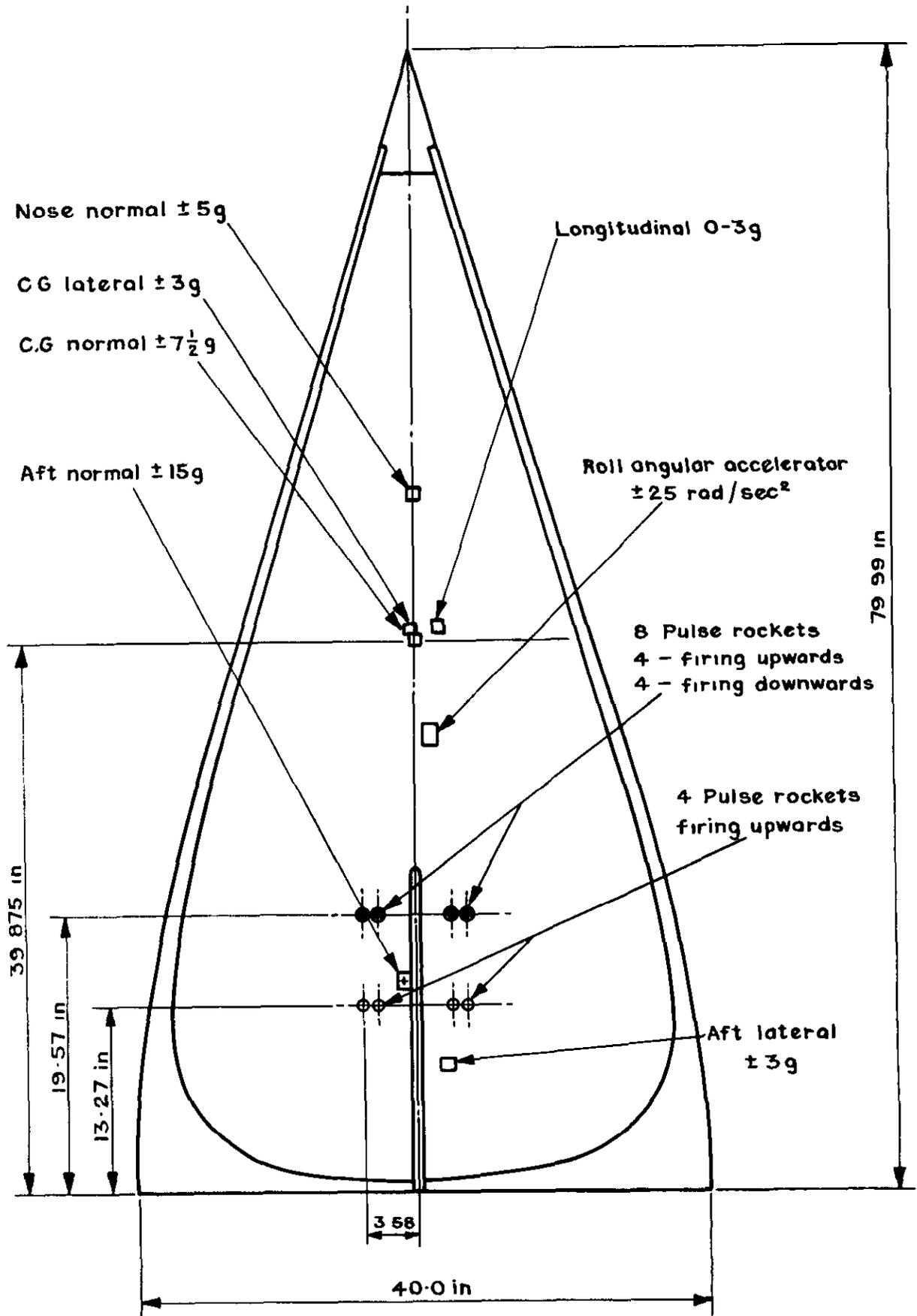
Fig. 12 Positions of accelerometers and pulse rockets
