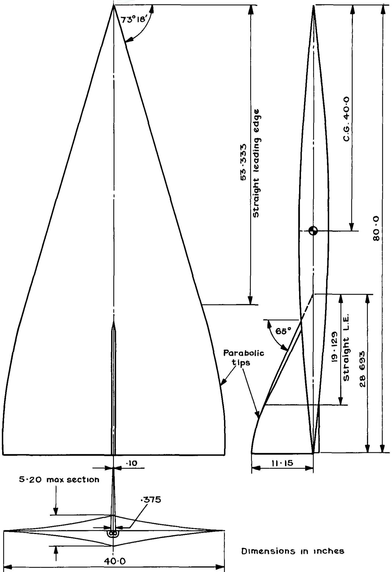
Fig.1 Model geometry
