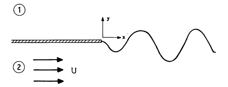
Vortex sheet leaving a plate and undergoing a spatial instability. In the unperturbed state the fluid in region 1 (above the plate) is stagnant, while that in region 2 (below the plate) streams with uniform velocity (U,0).
