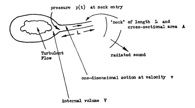
Fig. 1 Illustration of the model problem of sound generation by unsteady flow contained in a Helmholtz resonator
