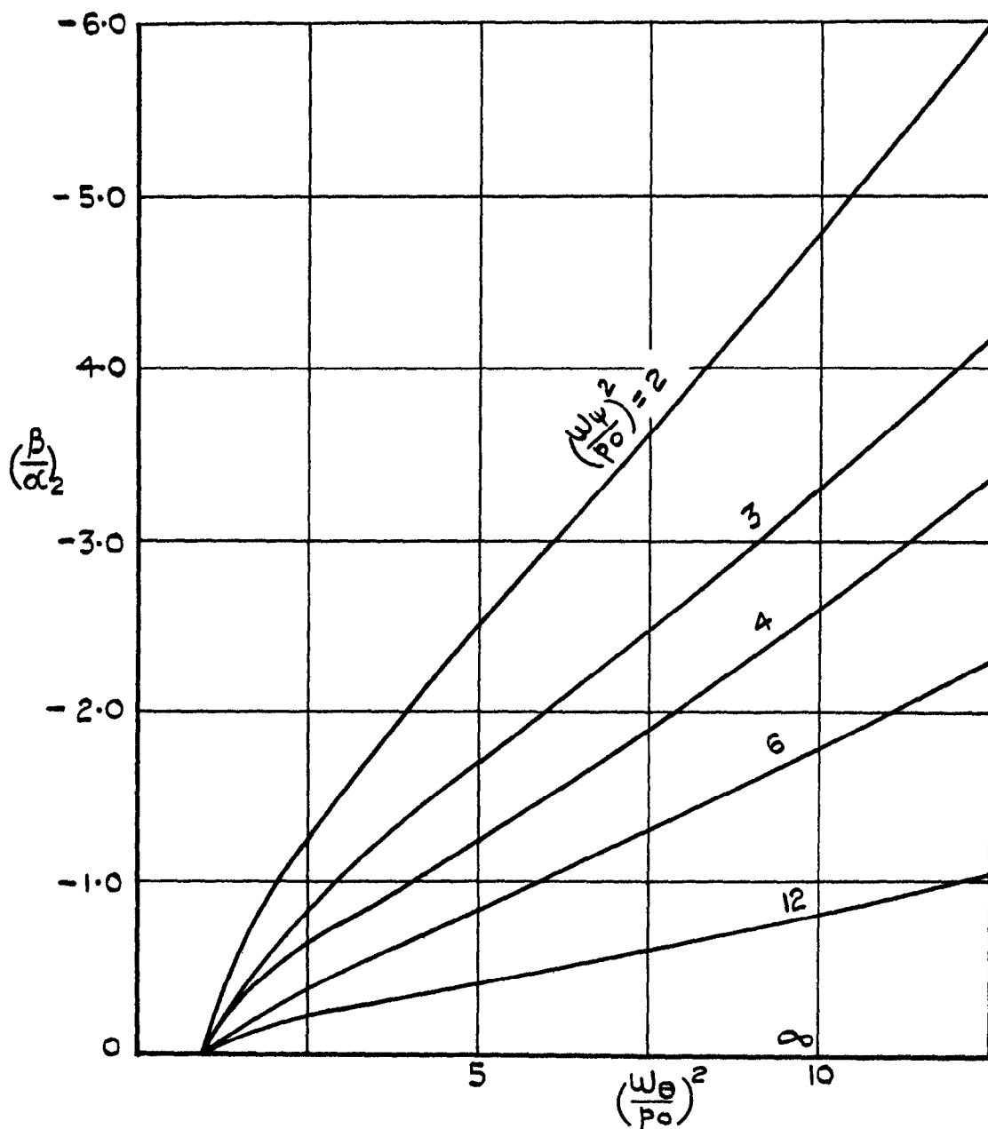
FIG. 41. AMPLITUDE RATIO \beta/\alpha OF THE LOW FREQUENCY OSCILLATION OF AN AIRCRAFT ROLLING WITH p=p_0 HAVING A \ll B .
