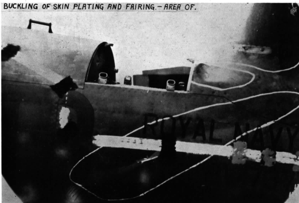
FIG. 14. External buckle on fuselage.
