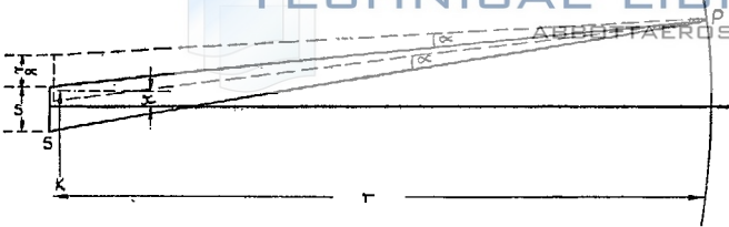
FIG. 7. Effect of errors on mirror surface.
