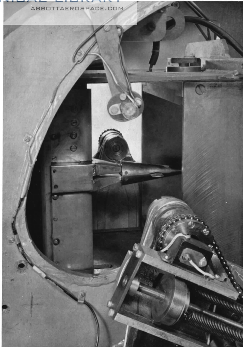
FIG. 6c. Duct side plate removed. Balance chamber showing balance, internal duct and shielding.
