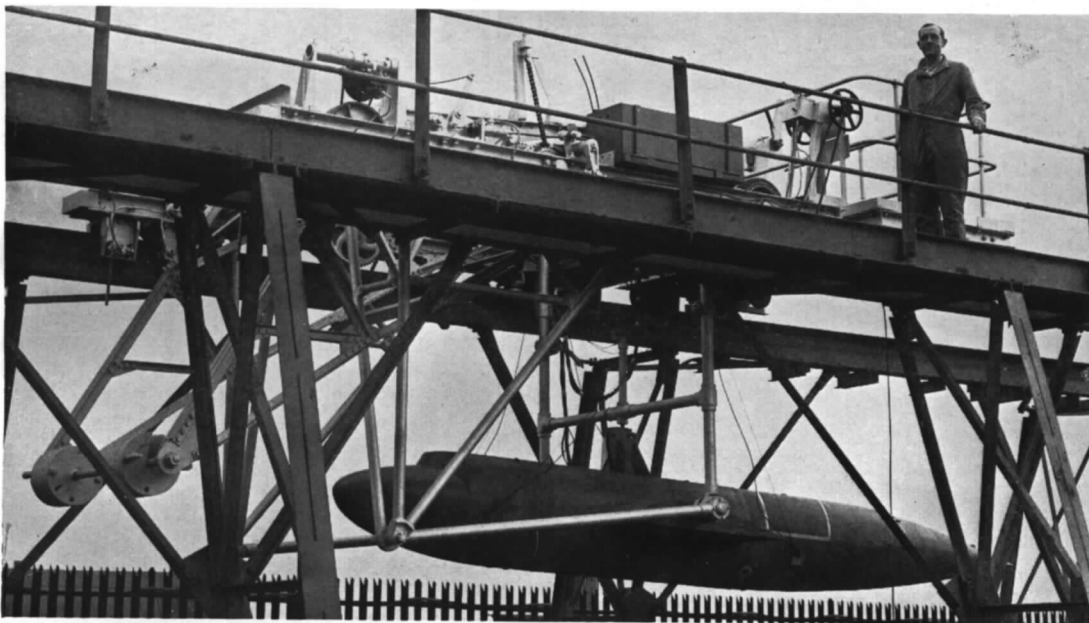
A ditching model on the carriage.
