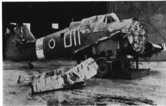
FIG. 19. Damage sustained by Martinet in ditching.
