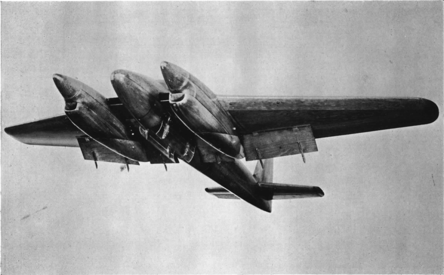
FIG. 5. Typical model of twin-engine bomber showing collapsible flaps and bomb doors. ( Sturgeon. )
