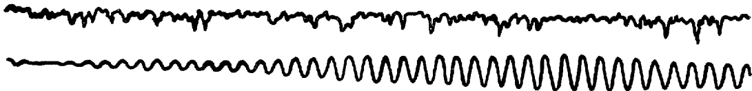
PHOTO. 8. Large-scale turbulence due to corner stall.
