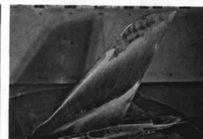
\alpha = 16 \text{ deg}, C_L = 0.91
