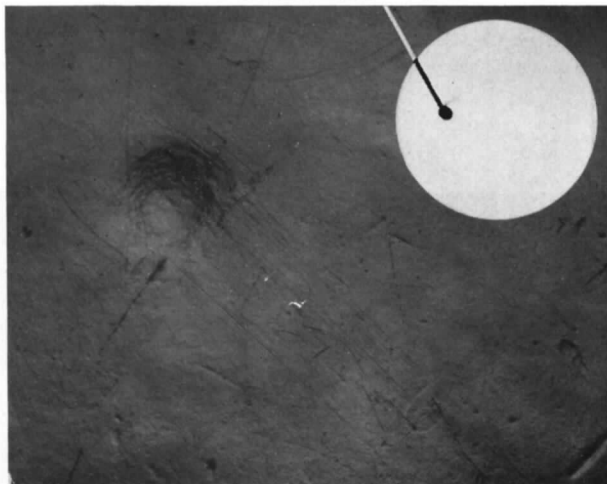
FIG. 20. Mark made on a \frac{1}{4} -in. thick aluminium specimen by a spherical 2\frac{1}{2} -mm diameter drop at 800 ft/sec.
