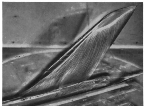
FIG. 9. Flow patterns, droop 'C'. R = 2.6 \times 10^6 , M = 0.27 (Section 3.1.2).
