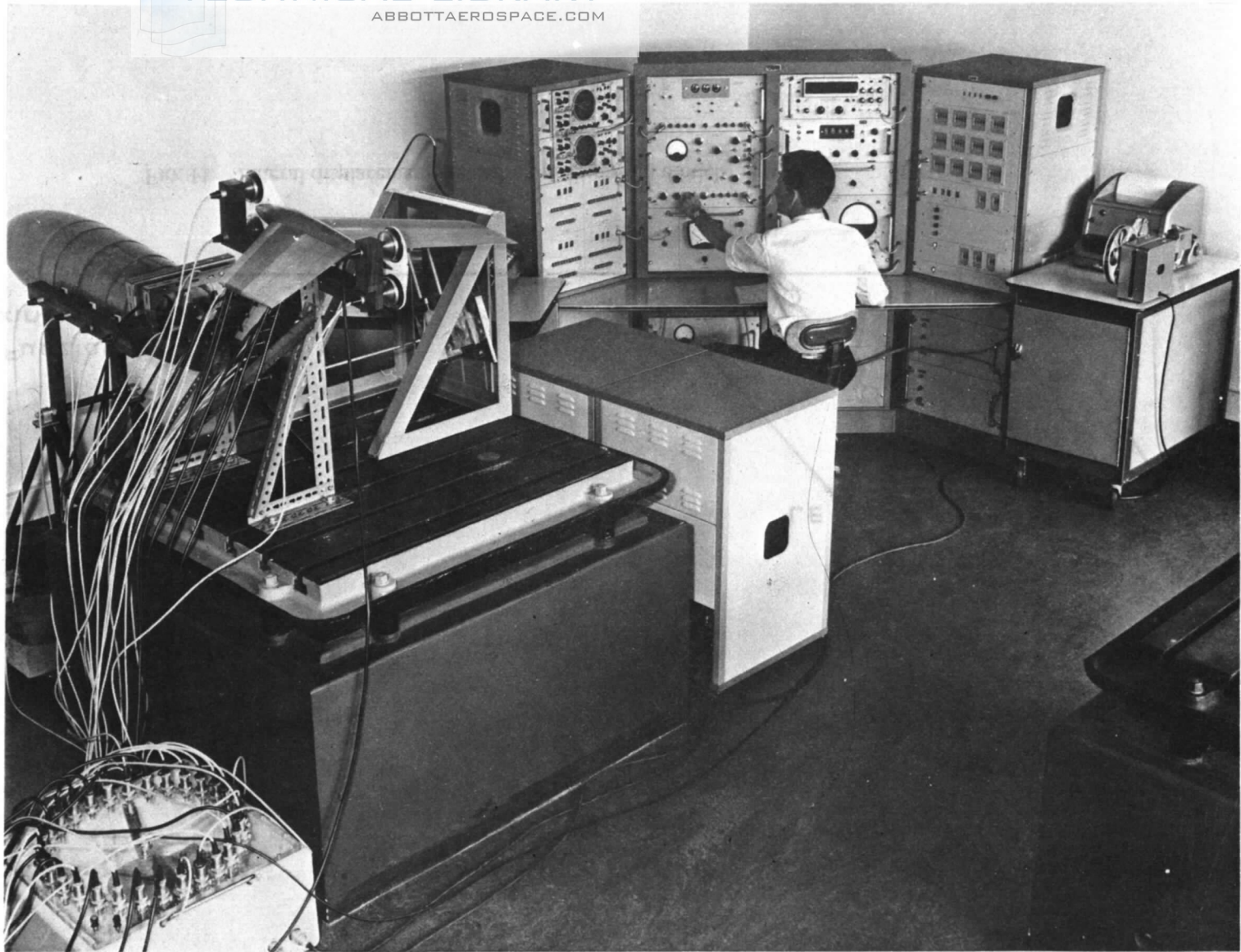
FIG. 10. Resonance testing of the flutter model.
