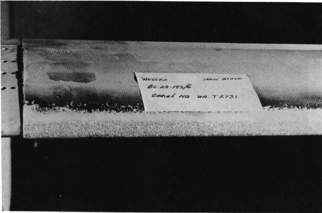
Heavy erosion of Wessex main blade (tip cap removed)
