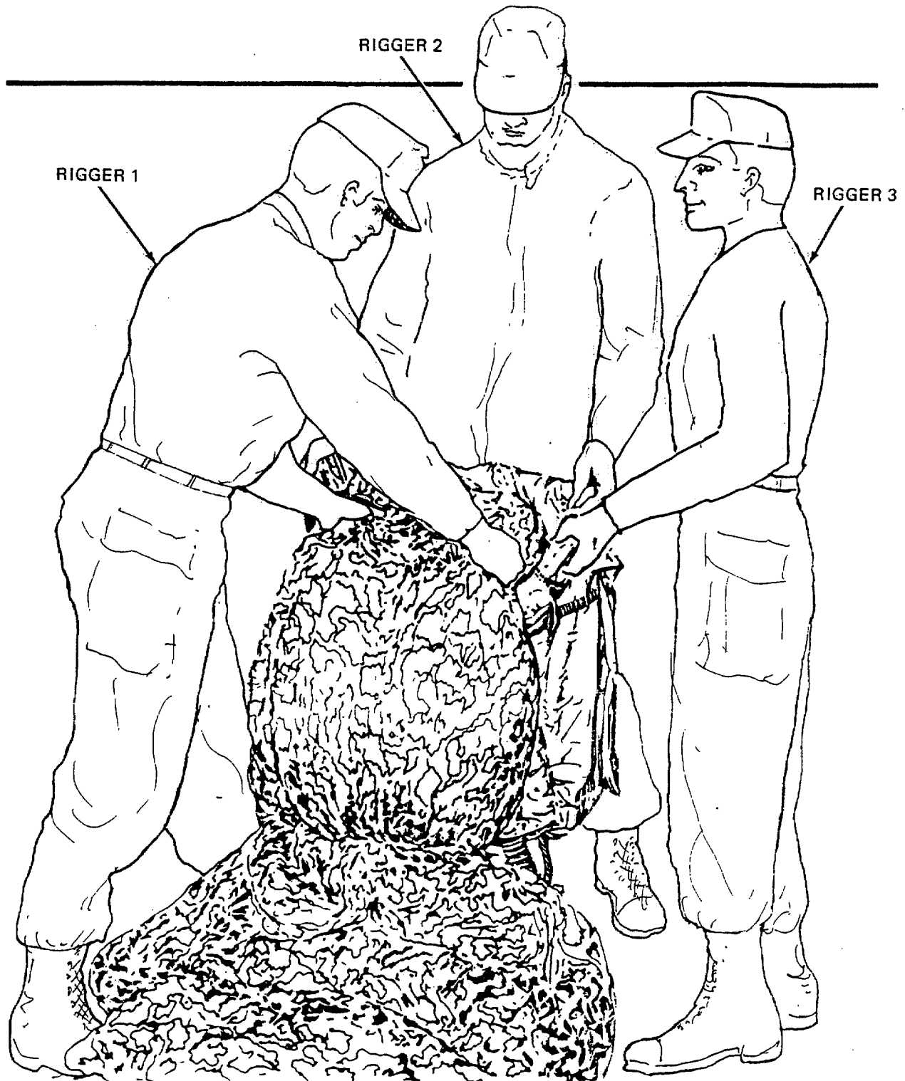
Figure 2-79. Stowing the Canopy Into the Deployment Bag .
