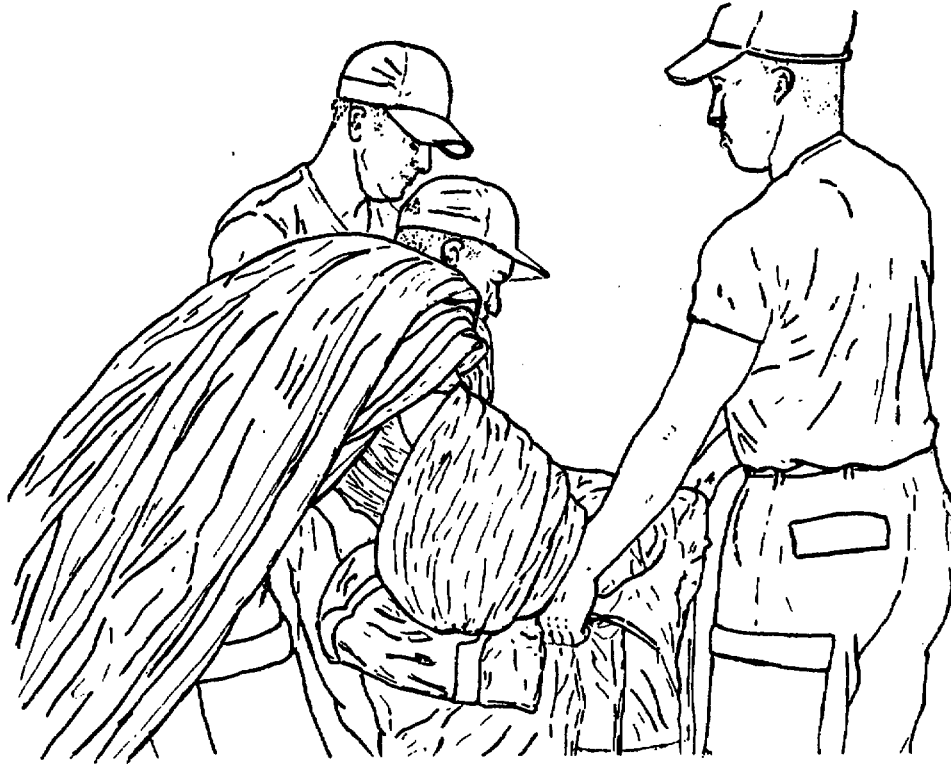
Figure 2-30. Stowing the Canopy in Deployment Bag.
