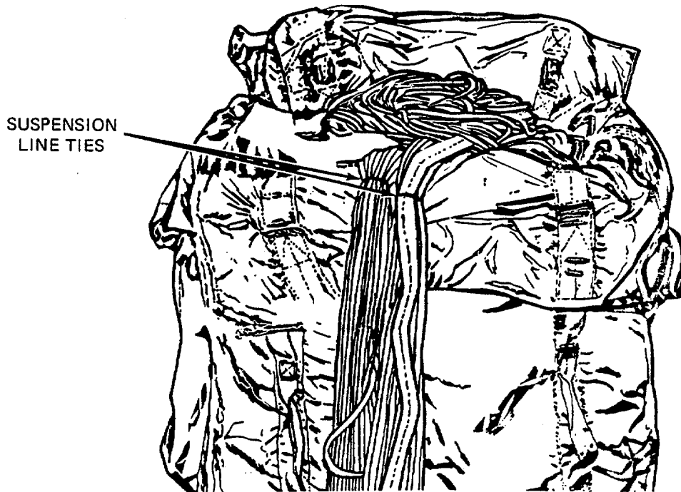
Figure 2-81. S-Folding Suspension Lines on Top of Stowed Canopy.
