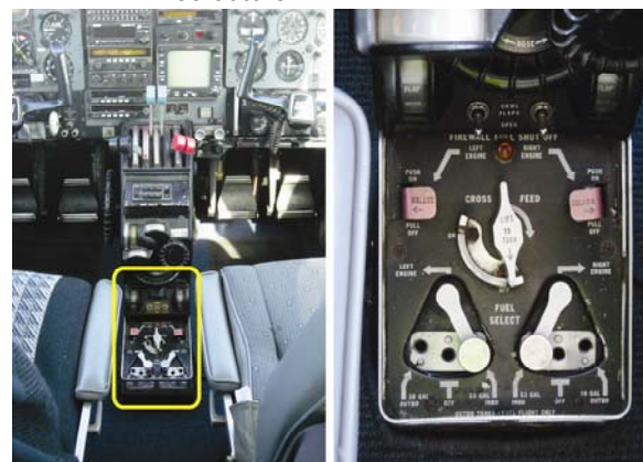
Figure 1: Central fuel control panel and fuel selectors in VH-ZMK
