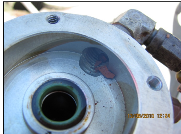
Figure 2: Fuel manifold valve with debris
