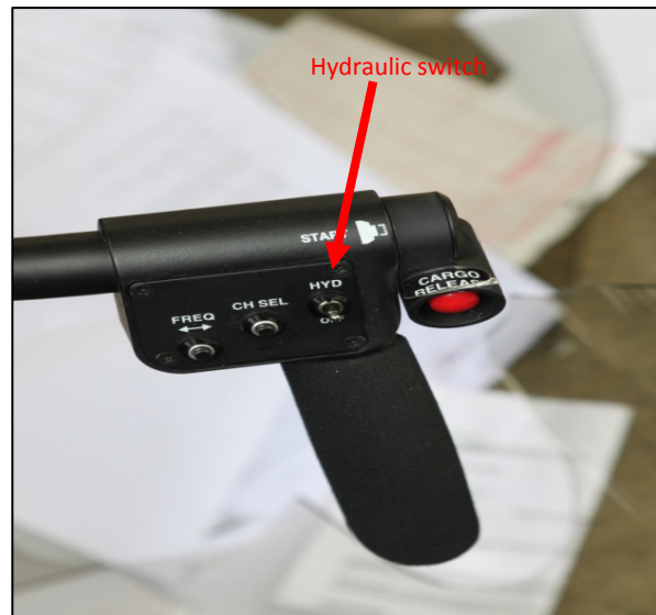
Figure 2: VH-ZVF Cyclic mounted hydraulic switch
