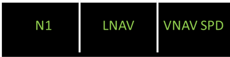
Figure 2: Representation of the FMA during climb in VNAV and LVL CHG modes
