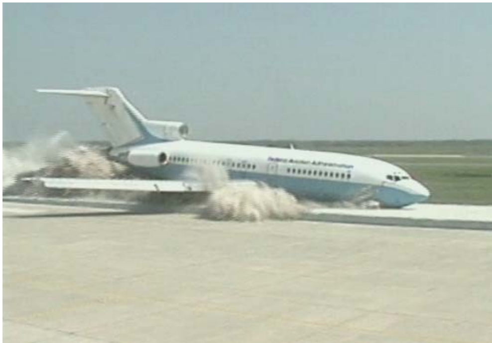
Figure 16: FAA performance trials of the EMAS system, simulating a runway overrun of a Boeing 727-200 aircraft
