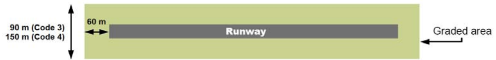
Figure 7: Required runway strip dimensions for non-instrument runways in Australia (fully graded area only)
