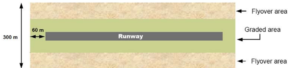
Figure 8: Required runway strip dimensions for instrument runways in Australia (both graded and flyover area)
