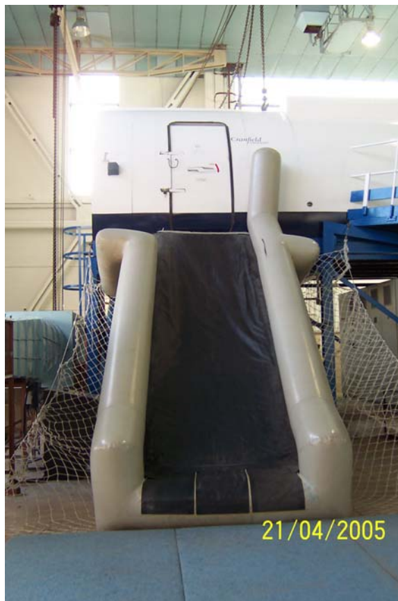
L4: Evacuation slide fitted to Boeing 737 Type I exit (photograph © Lauren Thomas 2005)
