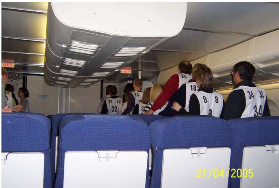
L10: Passengers evacuating, Large Cabin Evacuation Simulator (LCES) with dual-lane flow commands and half-height bulkheads (photograph © Lauren Thomas 2005)
