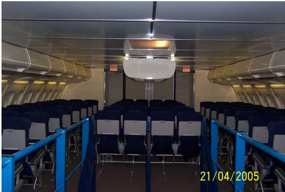
L7: Large Cabin Evacuation Simulator (LCES), upper deck view towards front of cabin, showing full-height bulkheads (photograph © Lauren Thomas 2005)
