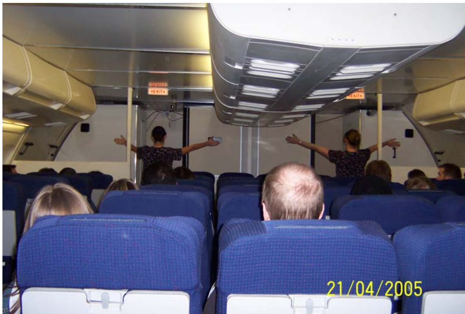
L8: Safety briefing in progress, Large Cabin Evacuation Simulator (LCES), showing half-height bulkheads (photograph © Lauren Thomas 2005)
