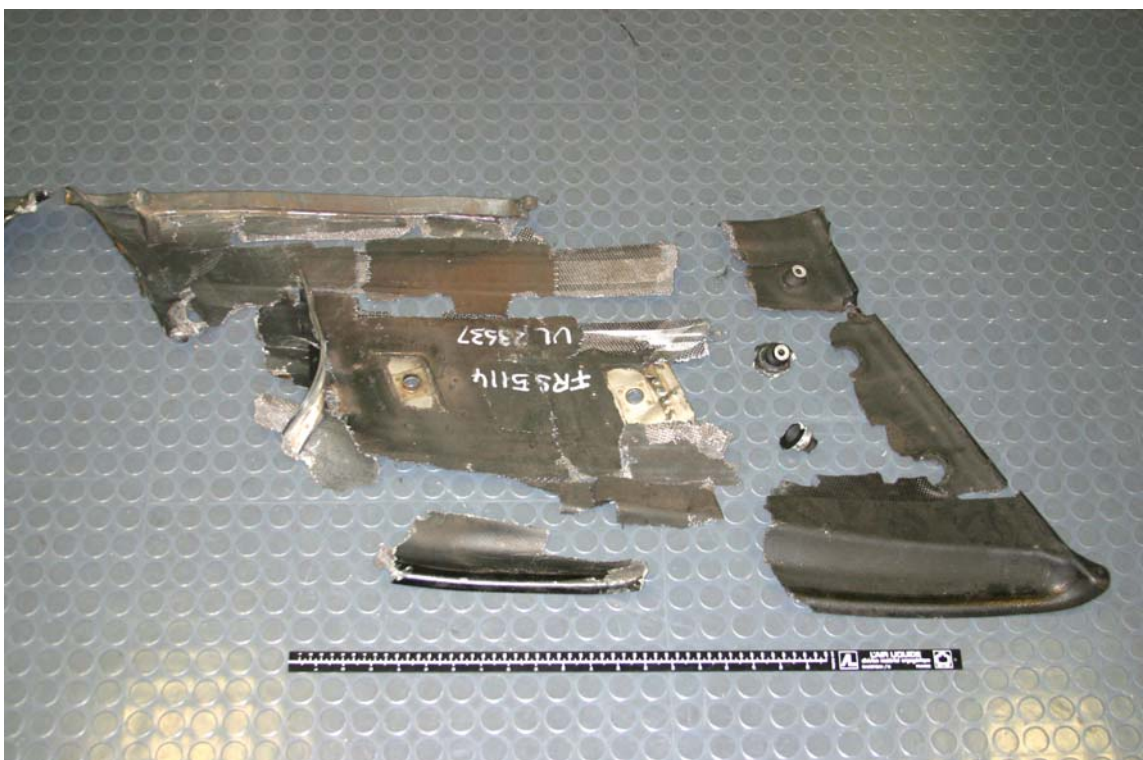
Figure 2. Received remnants of the INA drive fairing – side 2.
