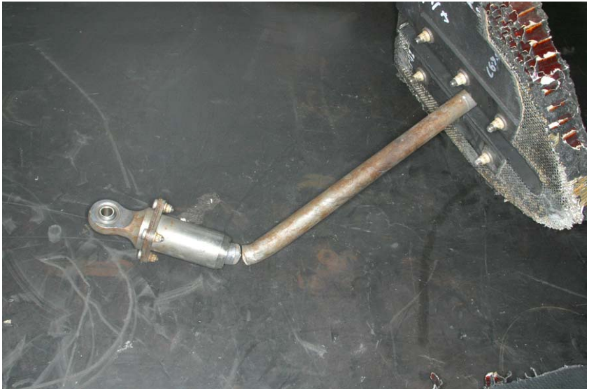
Figure 6. Blocker door actuator rod bending failure.
