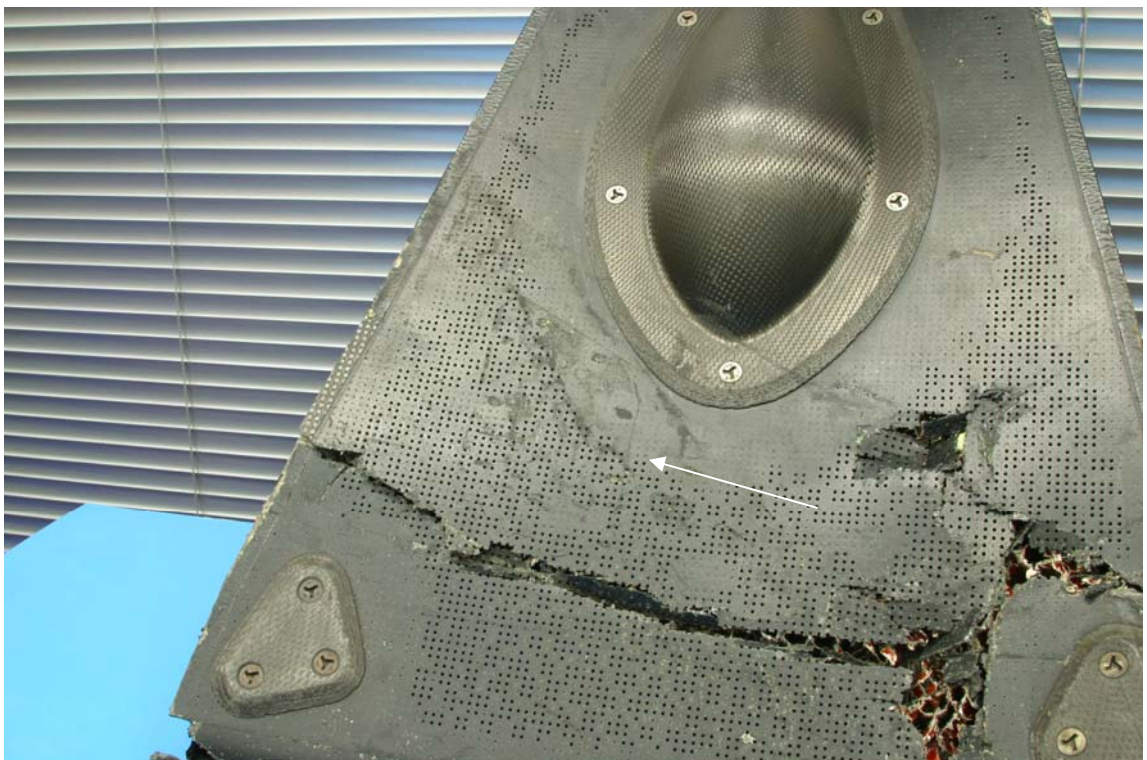
Figure 7. Inward facing surface of blocker door showing impact witness mark from a drive fairing panel (arrowed).
