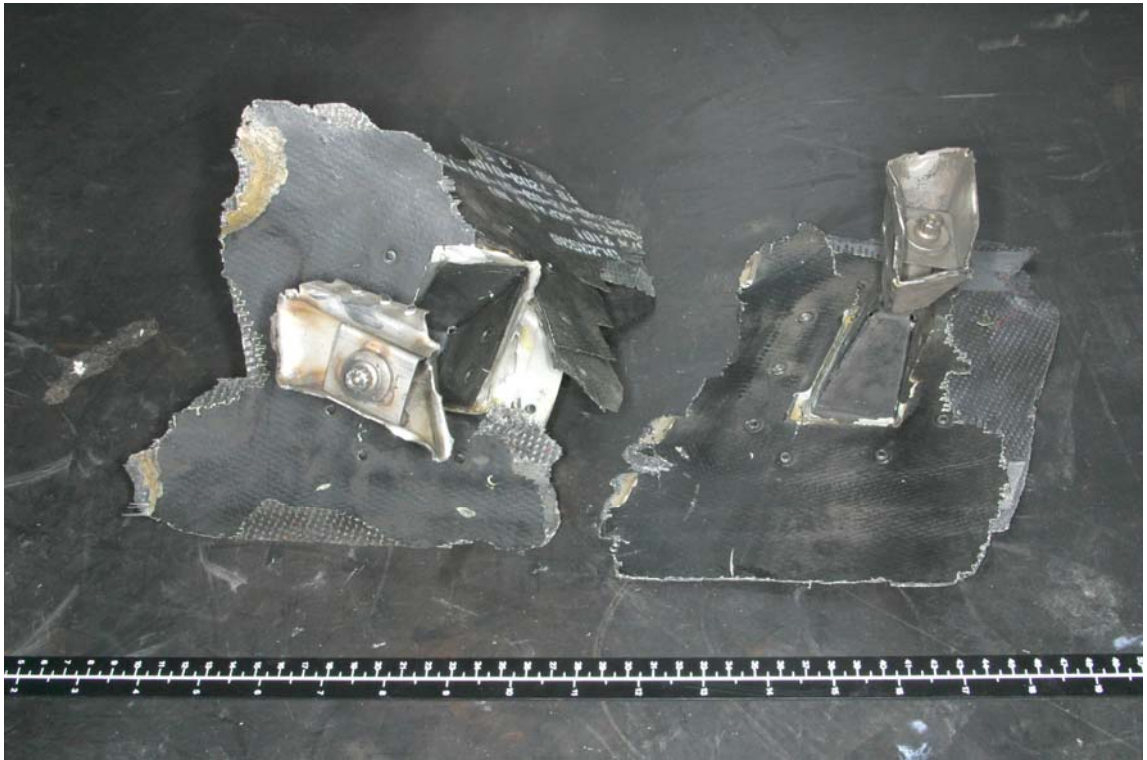
Figure 11. Separated drive fairing bolt towers.
