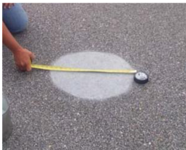
Sand Patch Test
