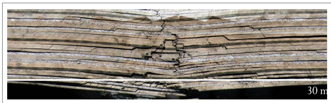
Figure 25 Section through 50 J, 20 mm impact on 33 ply painted, mesh covered laminate
