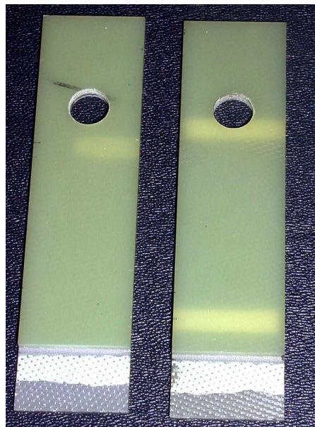
FIGURE 35. EXAMPLE OF FIRST-PLY FAILURE IN FIBERGLASS/EPOXY ASTM D 3165 SPECIMEN. THE FIRST-PLY OF LAMINATE CAN BE SEEN STILL ADHERING TO THE ADHESIVE ON BOTH PORTIONS OF THE SPECIMEN.
