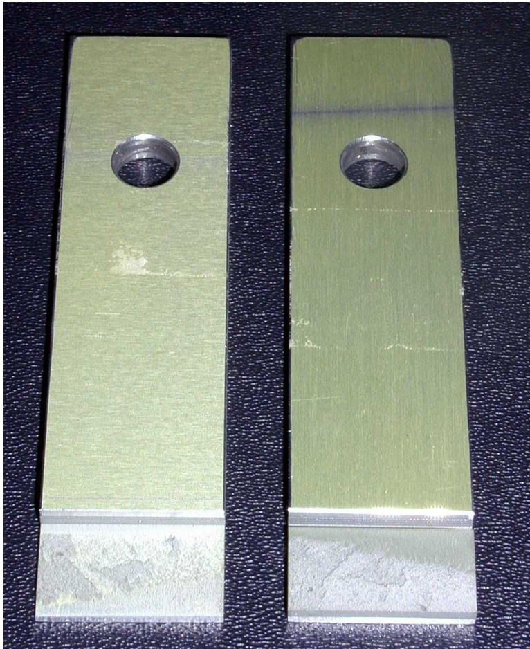
FIGURE 36. EXAMPLE OF COHESIVE/ADHESIVE FAILURE OF ALUMINUM ADHEREND ASTM D 3165 SPECIMEN. NOTE THE <50% ADHESIVE FAILURE ON THE UPPER PORTION OF THE RIGHT HALF OF SPECIMEN.
