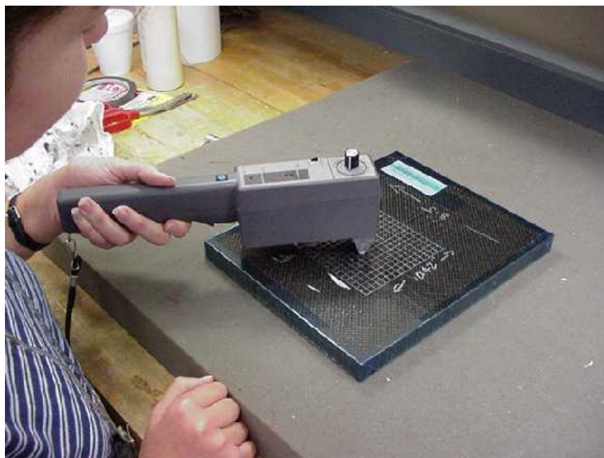
FIGURE 4-1. MITSUI WOODPECKER AUTOMATED TAP TESTER
