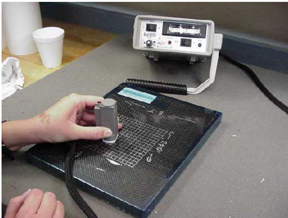
FIGURE 4-3. V-95 BOND TESTER USED FOR MECHANICAL IMPEDANCE ANALYSIS
