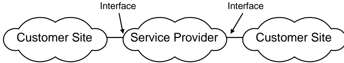
Figure 20. Interfaces Between Customer and Service Provider Networks
