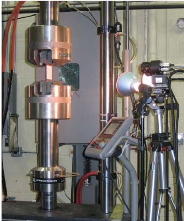
Figure 9. The MTS Servohydraulic Test Frame
