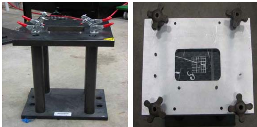
Figure 5. Support Fixture for CAI and TAI Impact Specimens
