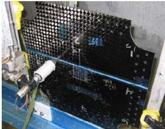
Figure 6. The TTU Scanning of PFS Test Specimen
