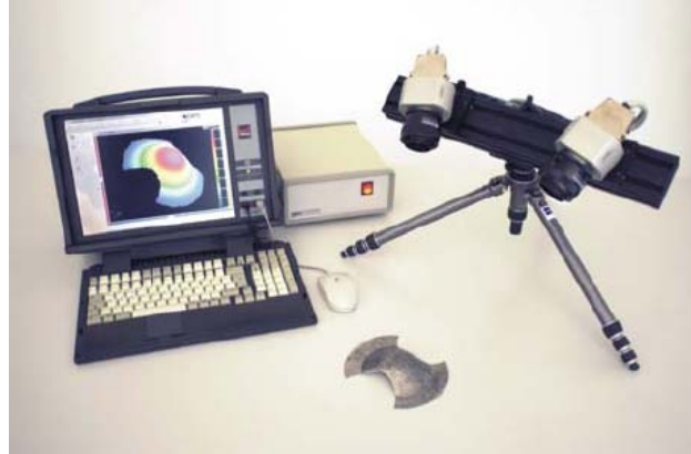
Figure 7. Portable Version of ARAMIS Photogrammetry System [40]
