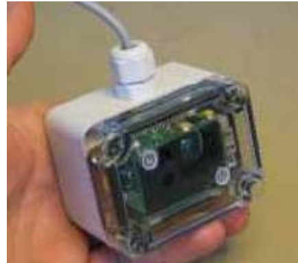
Figure A3- 2: Road Eye sensor
