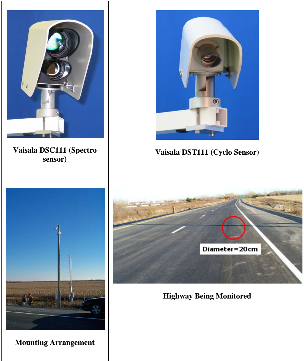
Figure 5.1: Vaisala Remote Road Surface State Sensor (Feng and Fu, 2008)
