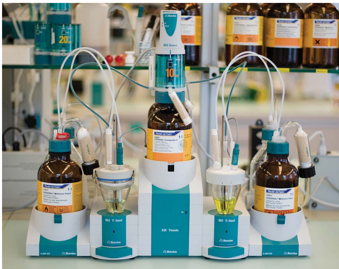
Figure 72: Setup for a water detection by a Karl-Fischer titration. (Image source: Wikipedia)
