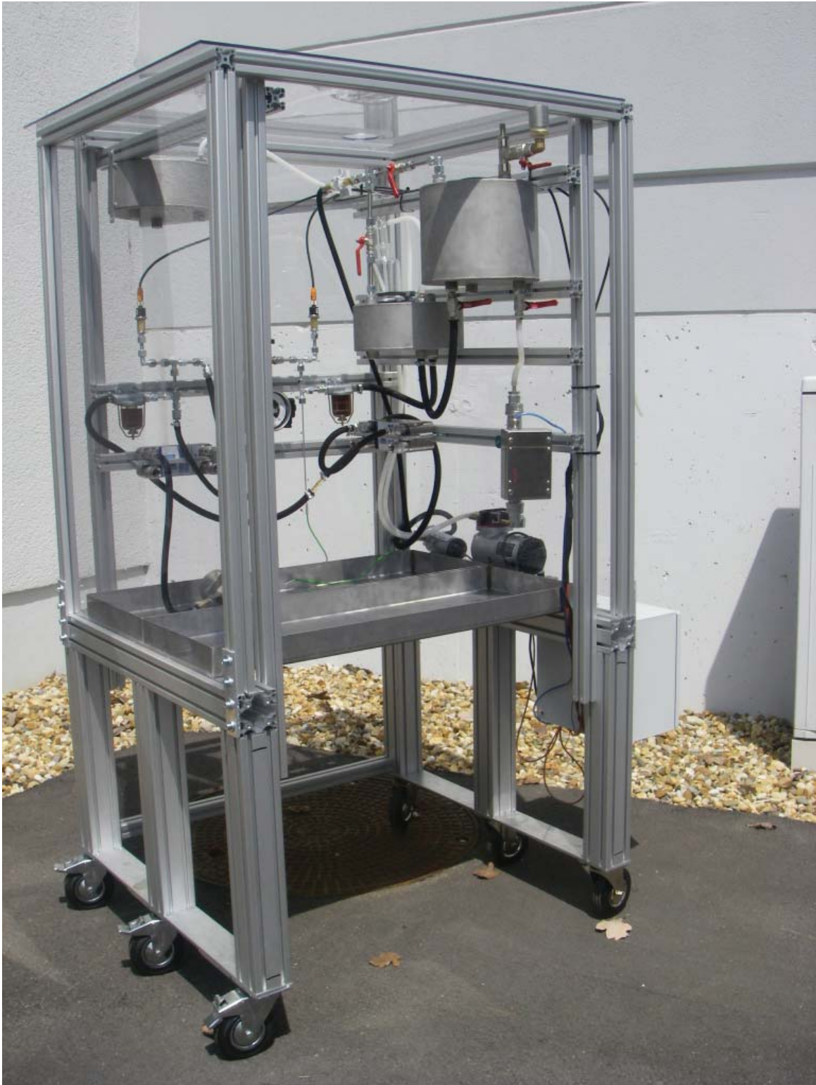
Figure 94: Actual vapour lock test rig with its fuel conditioning elements in place
