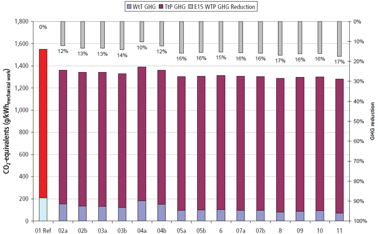
Figure 81: LBST well to propeller greenhouse gas emission analysis results, shown here as an example for the analysis of E-15 combustion.
