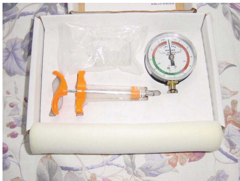
Figure 53: Hodges tester for gasoline volatility assessment.
