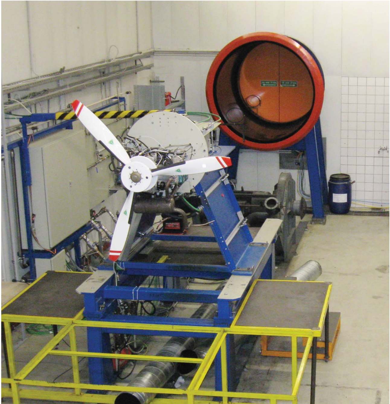
Figure 91: ROTAX 912 ULS on test rig
