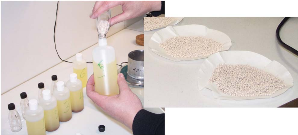
Figure 74: Zeolite water absorption experiment: Zeolite granules are given to gasoline probes (left). After vigorous shaking the zeolite is filtered, and the filter residues are weighed after some time of gasoline evaporative drying. Image right shows slightly differently coloured filtering samples with differing dry times.
