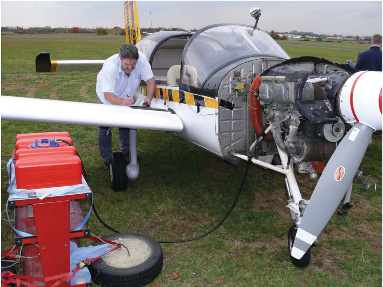
Figure 39: Morane icing test setup for operation with ethanol admixed fuels. The different gasoline compositions are taken from respective auxiliary tanks (red, left). They are fed by a bypass hose directly into the carburettor feed line. The aircraft is tied down to the ground with a strong rammed-in pole that is capable of supporting the full-power thrust of the engine.
