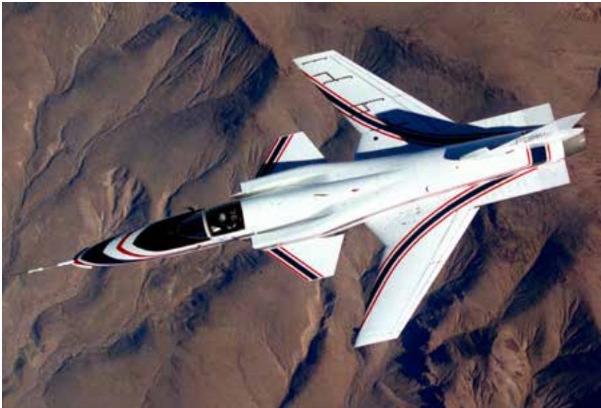
The first Grumman X-29A FSW demonstrator in flight over the Edwards range, 1985. (NASA)
