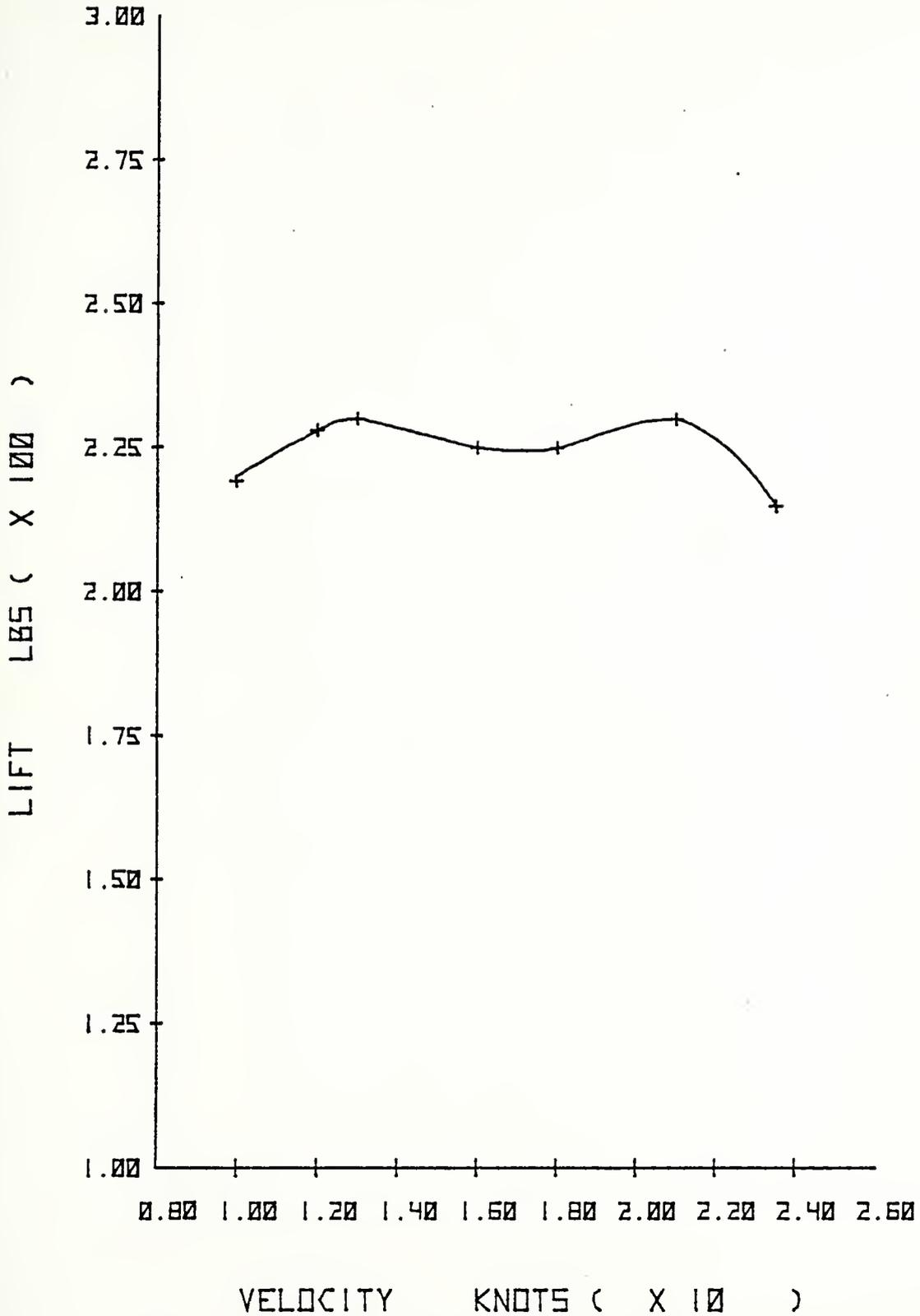
Figure 22. LIFT VS VELOCITY - BOW SEAL SHAPE 9980
