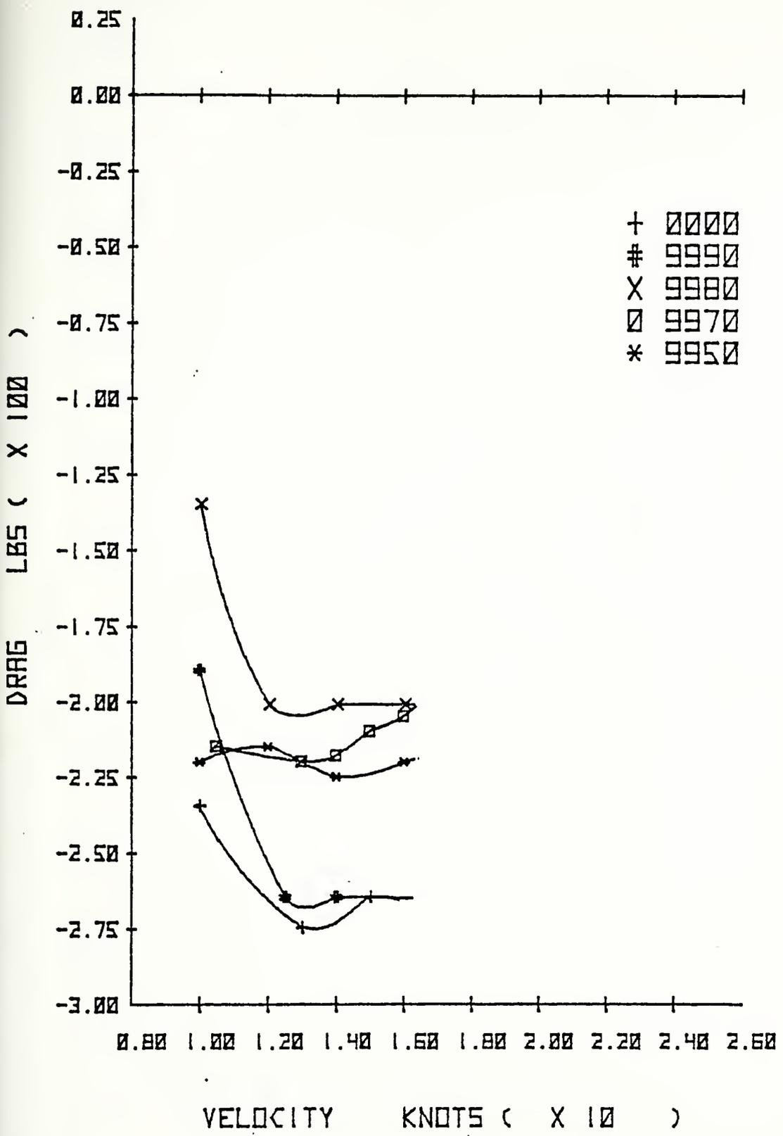
Figure 17. SUMMARY OF DRAG VS VELOCITY BELOW 17 KNOTS
