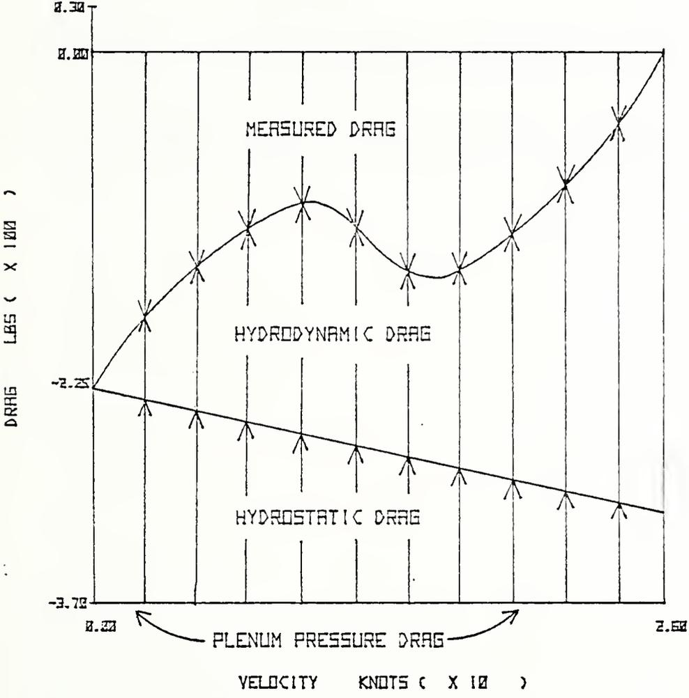
Typical Bow Seal Drag vs Velocity Curve
