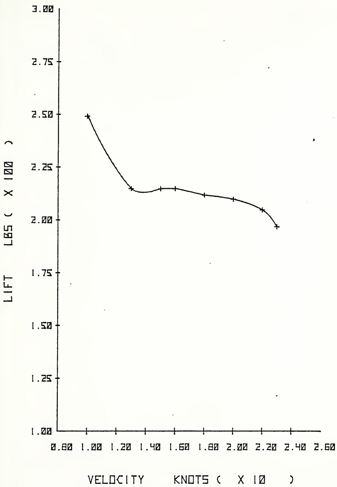
Figure 23. LIFT VS VELOCITY - BOW SEAL SHAPE 9970
