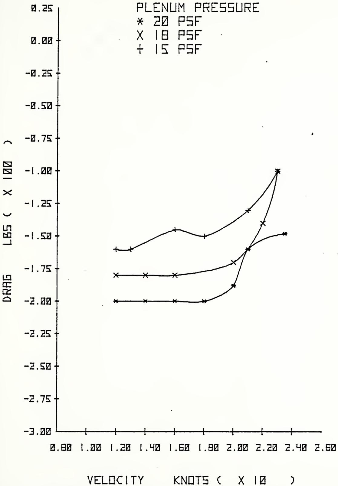
Figure 19. DRAG VS VELOCITY FOR VARYING PLENUM PRESSURES
