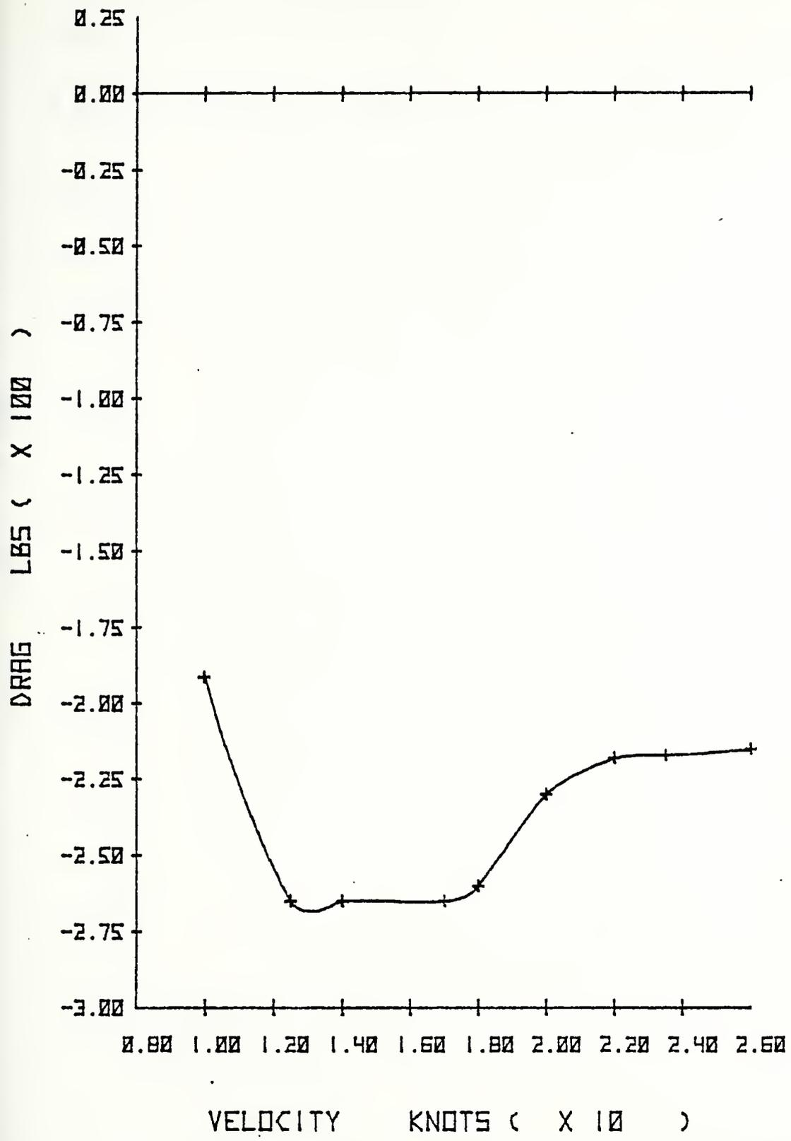
Figure 13. DRAG VS VELOCITY - BOW SEAL SHAPE 9990
