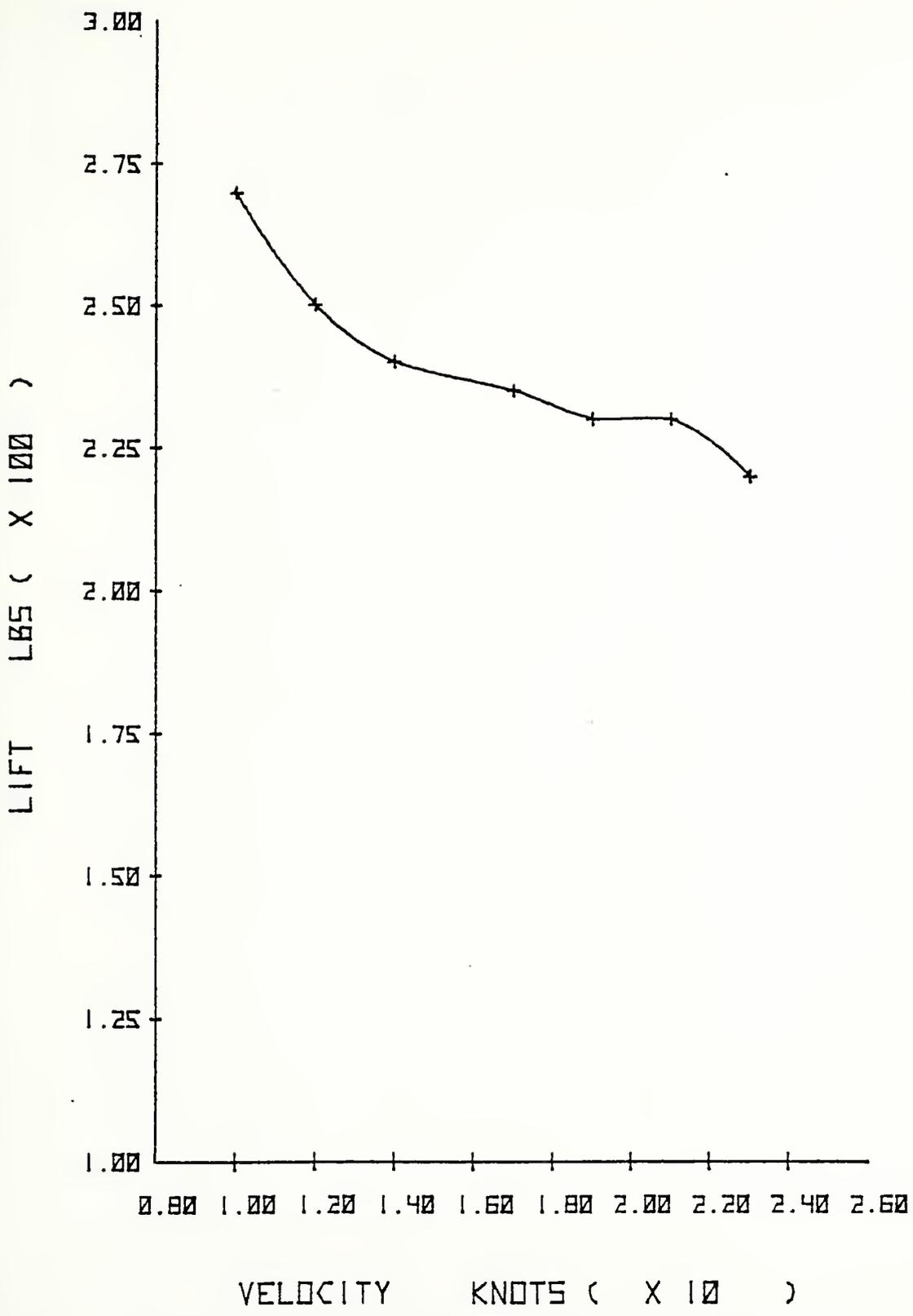
Figure 21. LIFT VS VELOCITY - BOW SEAL SHAPE 9990
