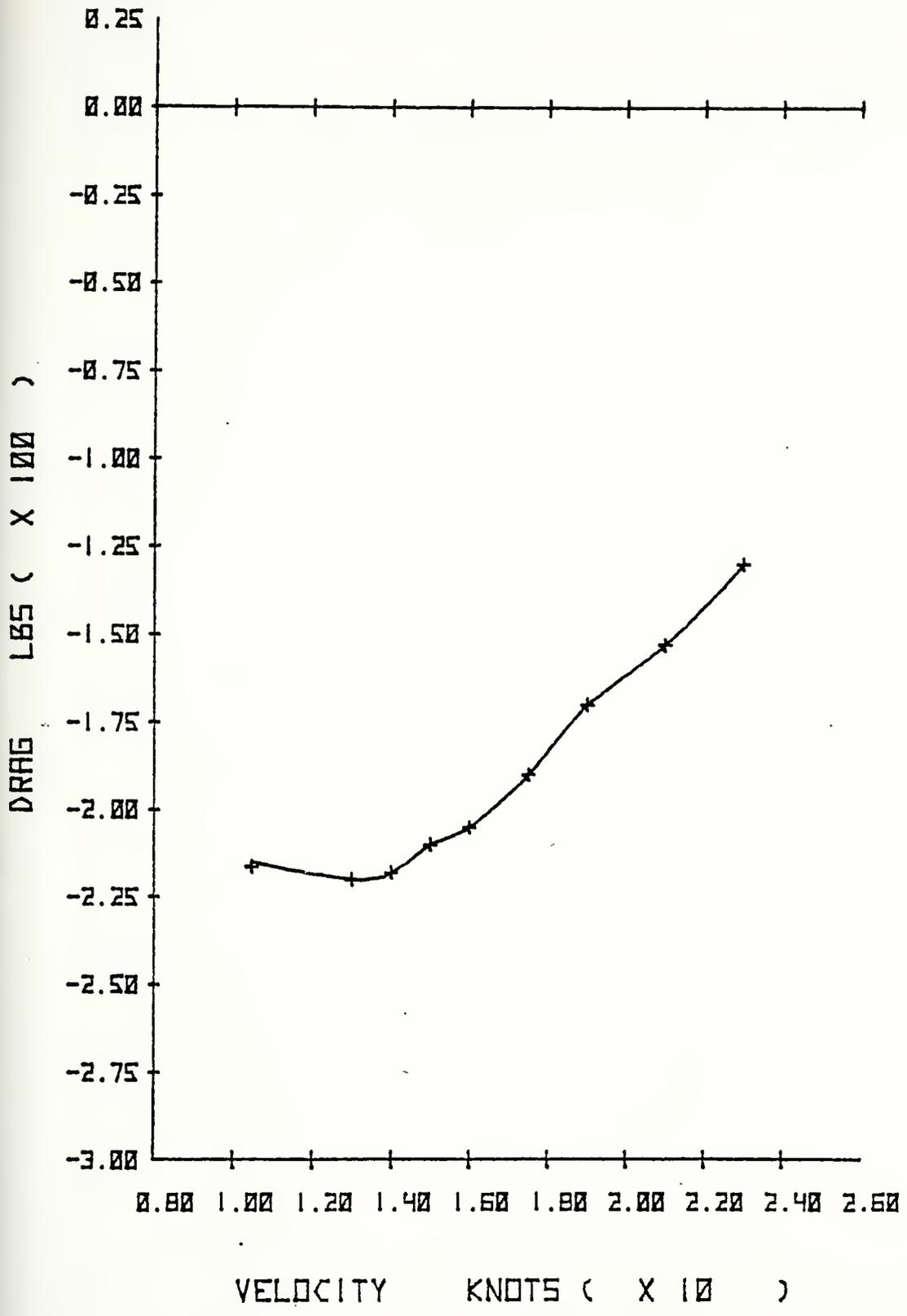
Figure 15. DRAG VS VELOCITY - BOW SEAL SHAPE 9970
