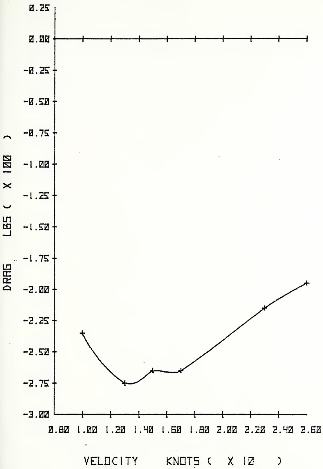
Figure 12. DRAG VS VELOCITY - BOW SEAL SHAPE 0000
