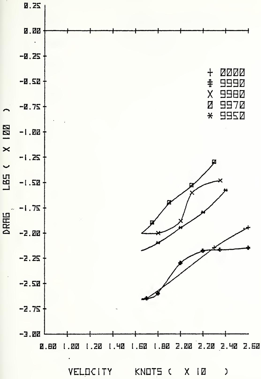
Figure 18. SUMMARY OF DRAG VS VELOCITY ABOVE 17 KNOTS
