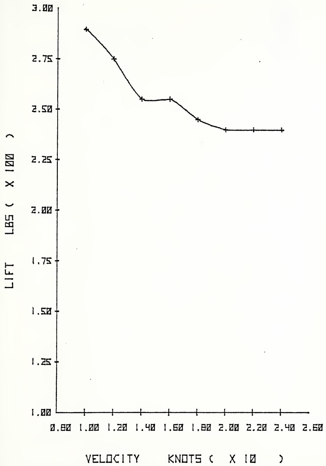
Figure 24. LIFT VS VELOCITY - BOW SEAL SHAPE 9950
