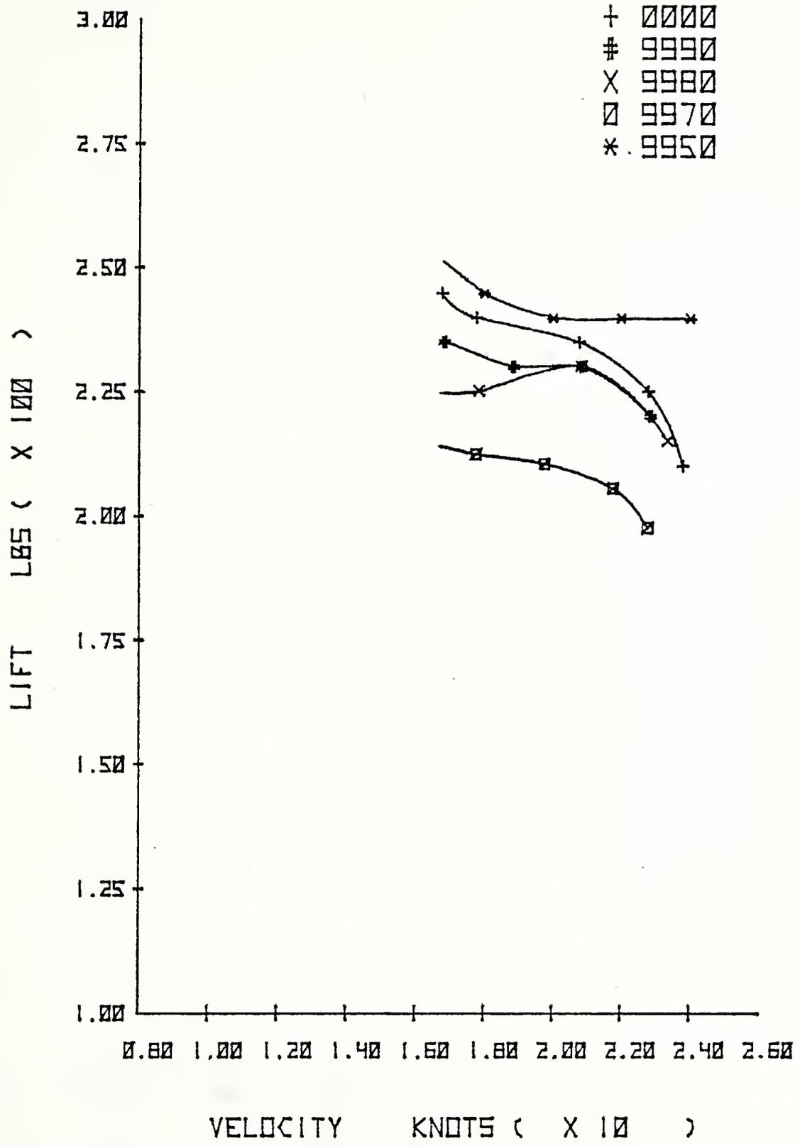
Figure 26. SUMMARY OF LIFT VS VELOCITY ABOVE 17 KNOTS
