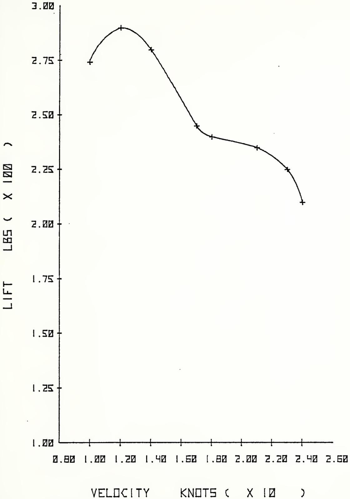
Figure 20. LIFT VS VELOCITY - BOW SEAL SHAPE 0000
