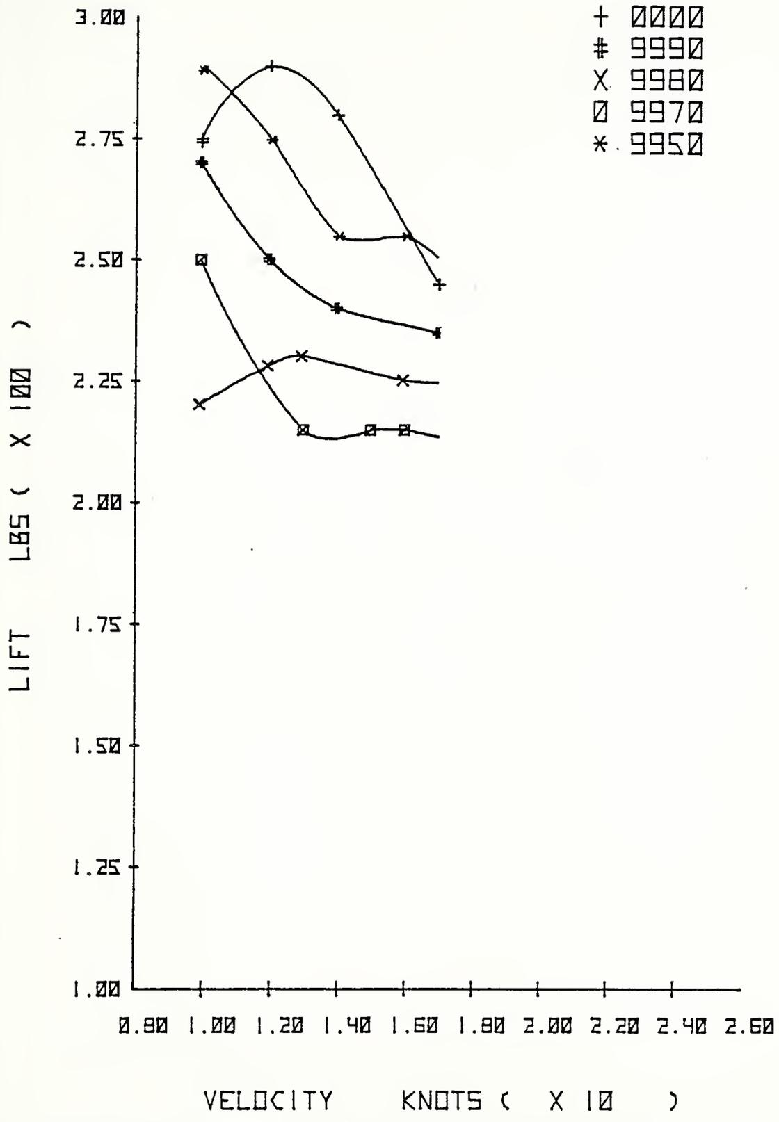
Figure 25. SUMMARY OF LIFT VS VELOCITY BELOW 17 KNOTS
