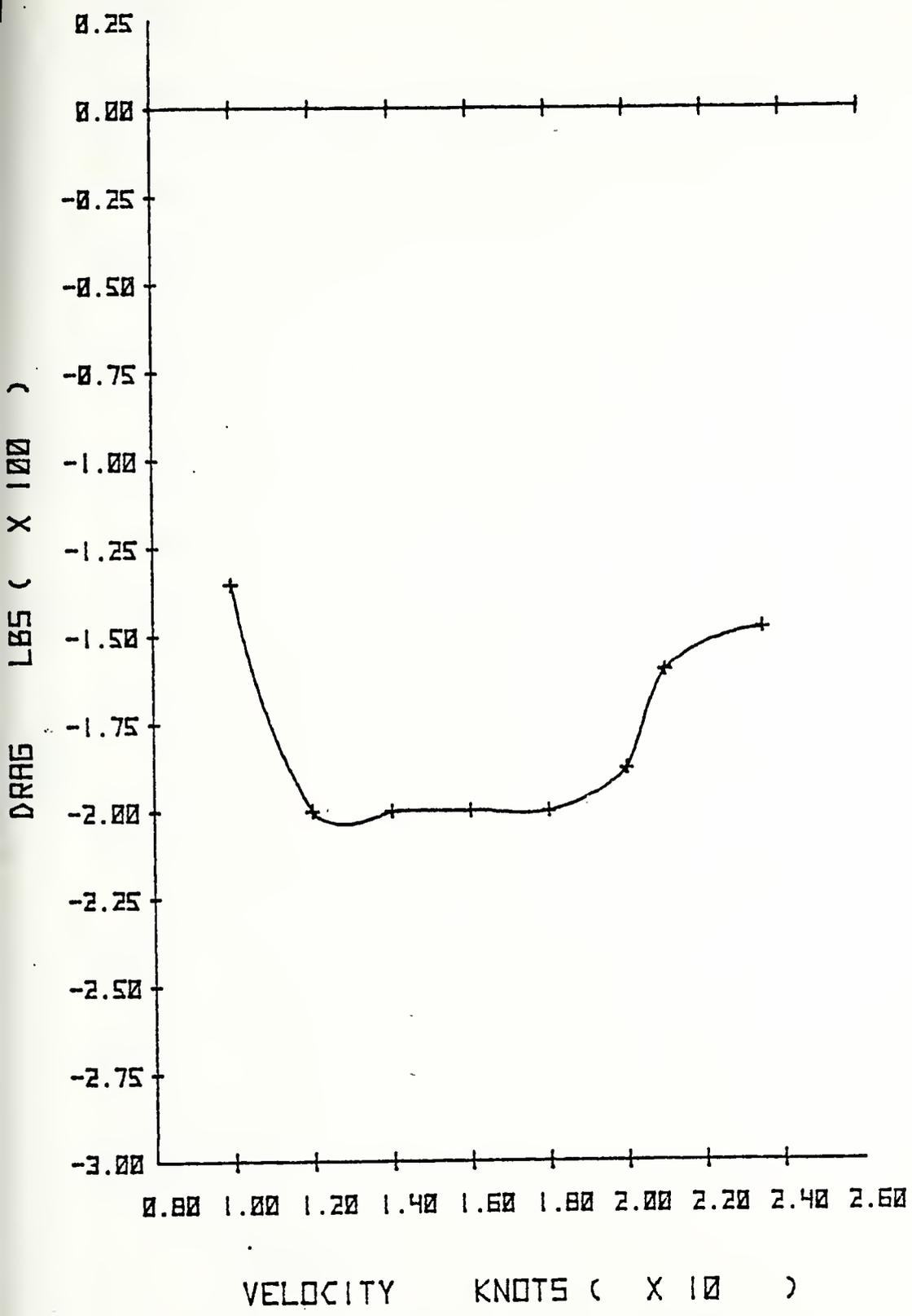
Figure 14. DRAG VS VELOCITY - BOW SEAL SHAPE 9980
