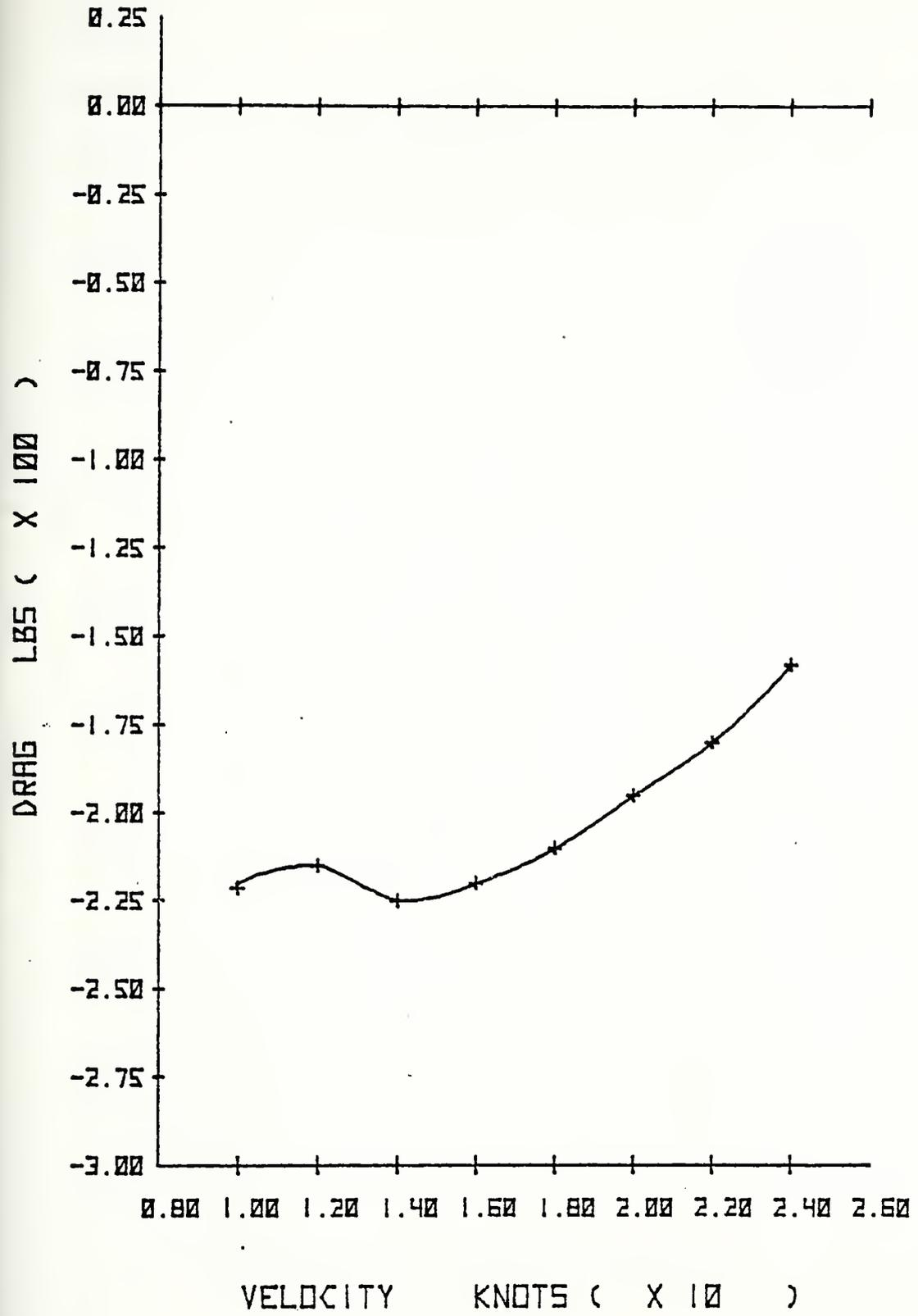
Figure 16. DRAG VS VELOCITY - BOW SEAL SHAPE 9950
