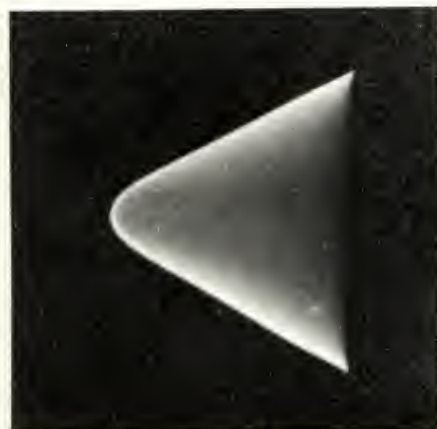
Run #90. 1 atm. V_{fa} 4.84 fps D_B 3/16 in.
