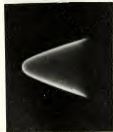
Run #93. 1/2 atm. V_{fa} 3.23 fps D_B 1/8 in.
