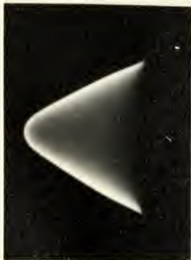
Run #88. Ethylene. 1/2 atm. V_{fa} 4.36 fps.
