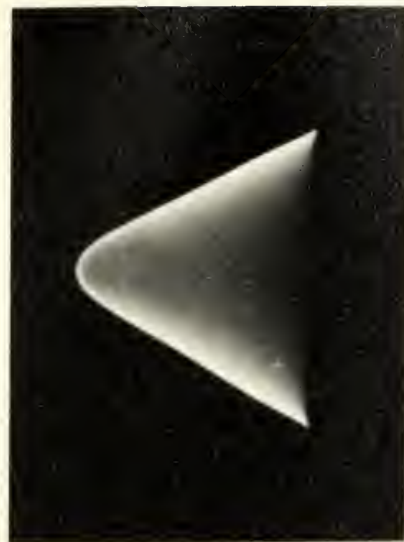
Run #90. Ethylene. 1 atm. V_{fa} 4.84 fps.
