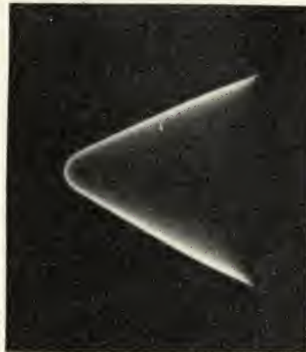
Run #81. Propane. 3/4 atm. V_{fa} 2.98 fps.
