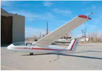
Blaik L-23 sailplane with microphone on left wingtip and installed recording equipment. (NASA)
