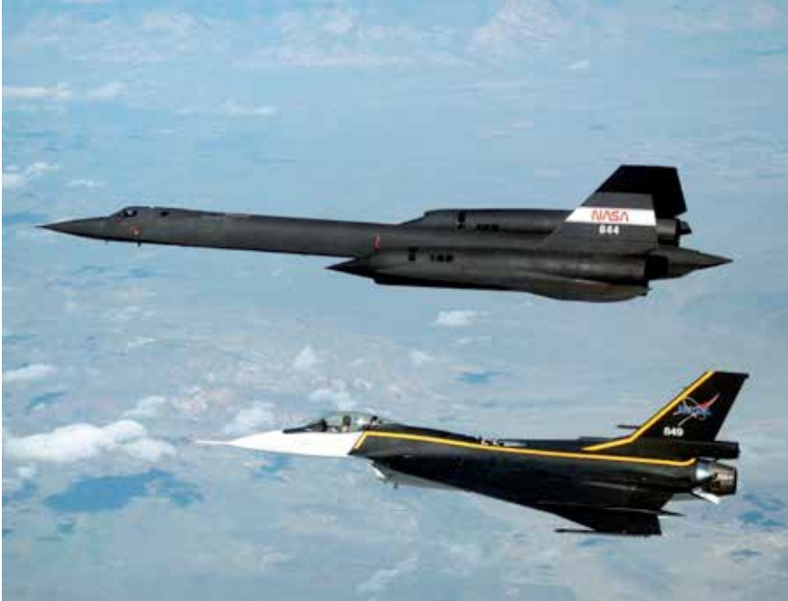
F-16XL and SR-71 during in-flight shock wave measurements in 1995. (NASA)
