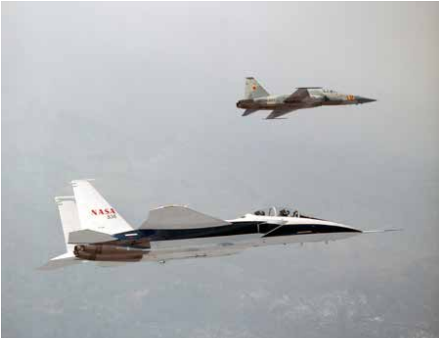
NASA F-15B and Navy F-5E during Inlet Spillage Shock Measurement Test, February 2002. (NASA)
