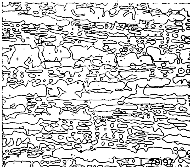
FIGURE 10.—Alloy 443 containing 25 percent cobalt, 25 percent nickel, and 50 percent molybdenum. Etched according to procedure 4 but stain omitted; alpha phase arranged in banded dendritic pattern in matrix of mu phase; X250.
