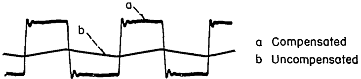
FIGURE 26.—Effect of compensation at high frequency. Time constant, 0.4 millisecond; square-wave frequency, 5,000 cycles per second.
