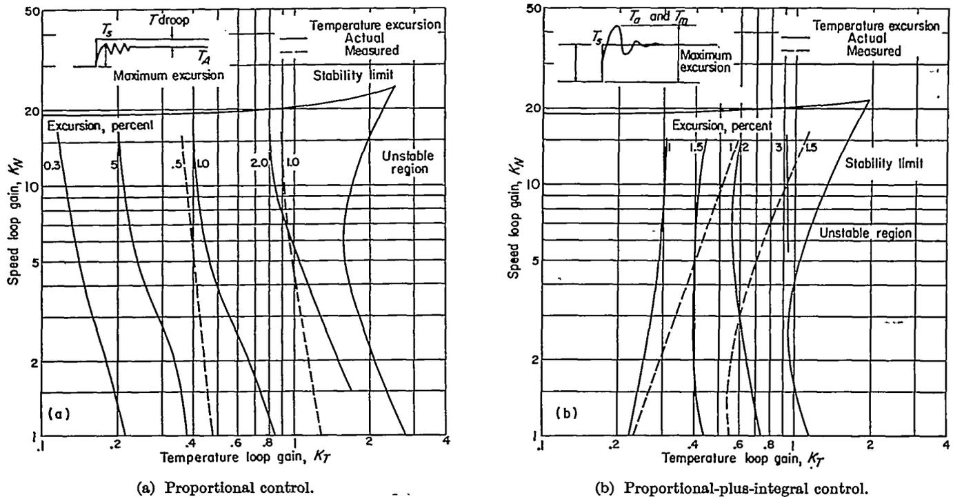
FIGURE 8.—Contour lines of actual and measured temperature excursions on stability limit map.
