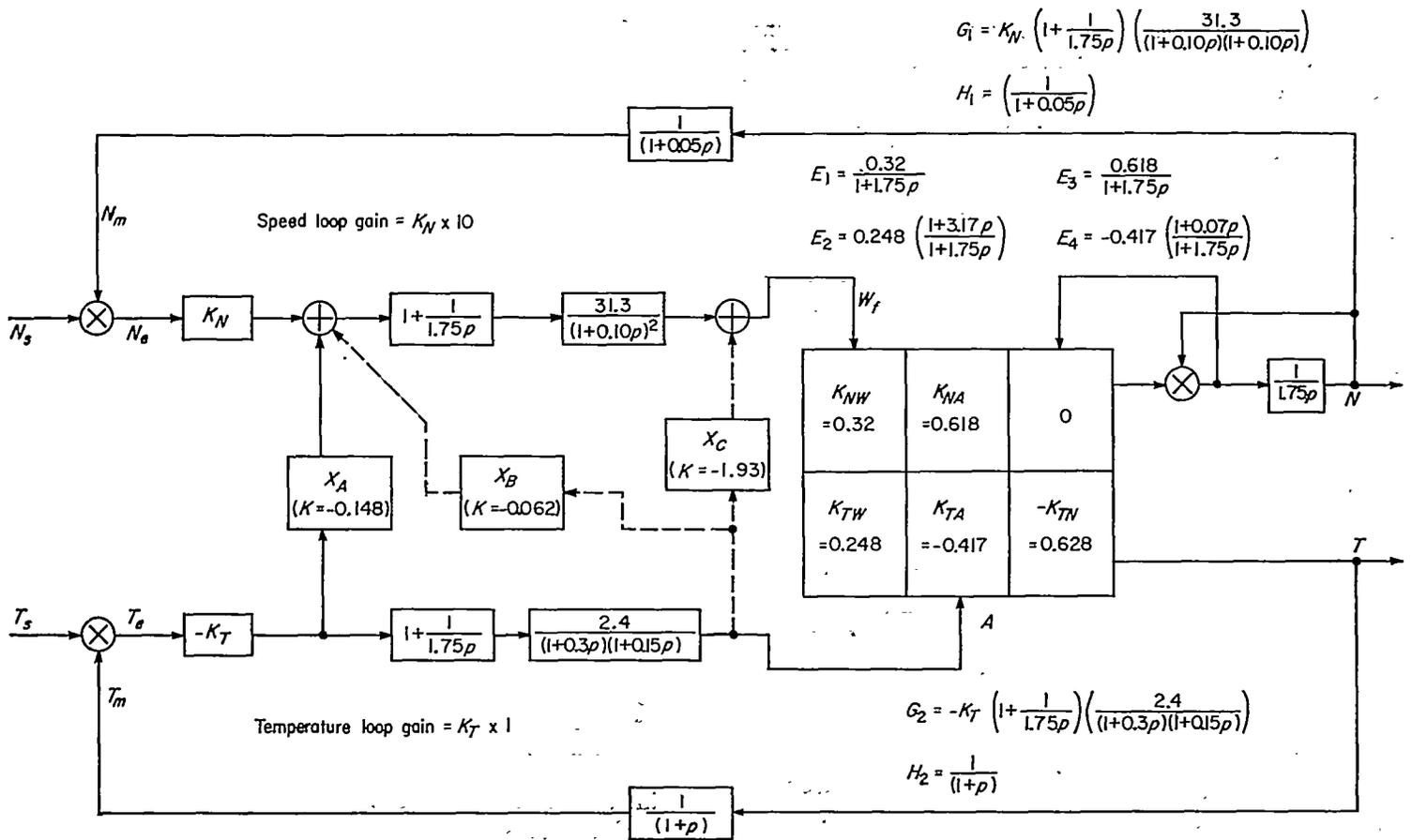
Figure 2.—Block diagram of system on analog computer.
