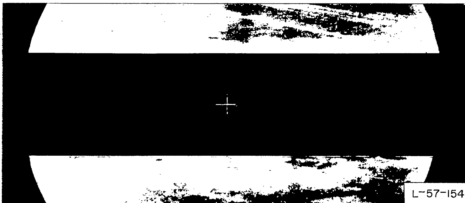
(g) Flash schlieren; R_x/x = 0.23 \times 10^6 per inch; X_{LE} = -18.0 inches; t = 0.003 to 0.005 inch.
