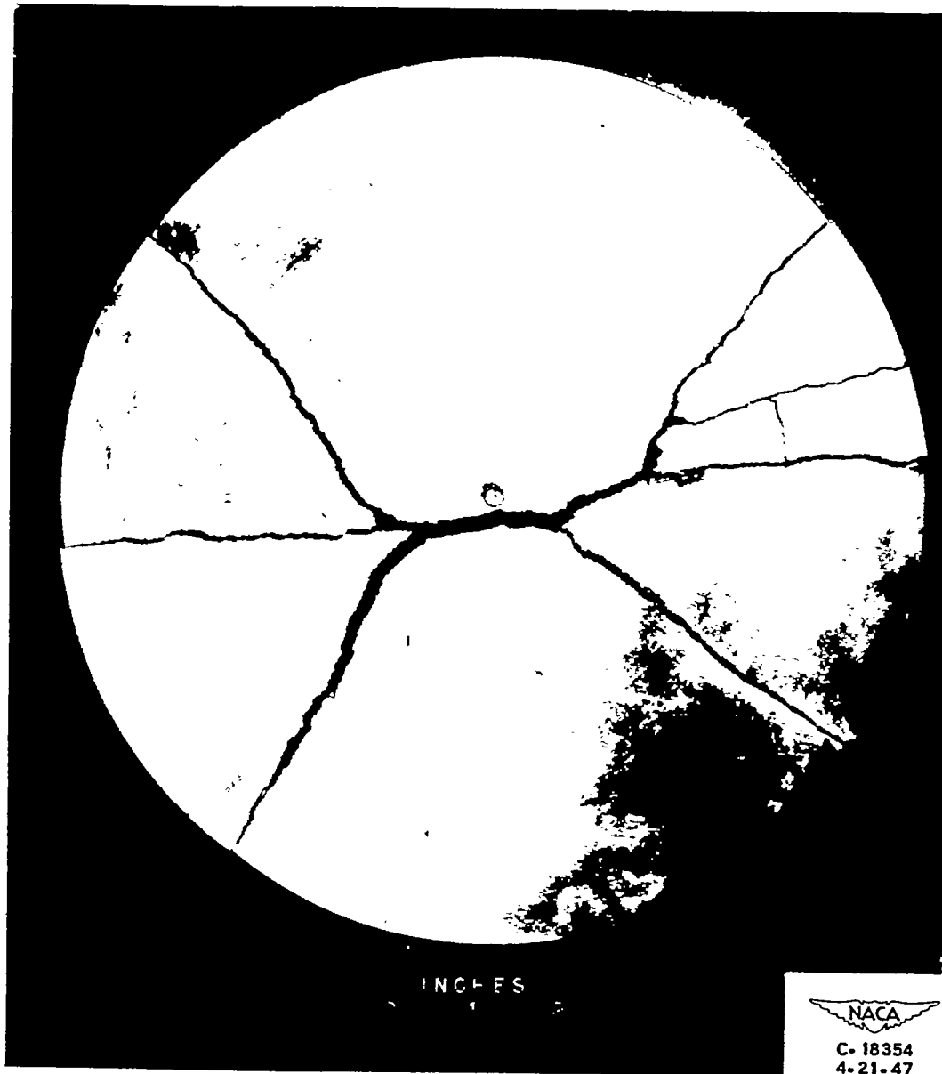
(e) Steel disk, SAE 1078. Reduction in diameter of tensile specimen in nonnecked region, 4.52 percent.
