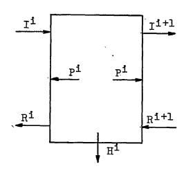
As in references 1 and 2, the absorber is considered as being arbitrarily divided into n convenient stations normal to the path of the radiation. Radiation of power I<sup>1</sup> from the (i-1)<sup>th</sup> station is incident upon the i<sup>th</sup> station of the absorber; whereas radiation R<sup>1</sup> from the i<sup>th</sup> station is incident upon the (i-1)<sup>th</sup> station.
