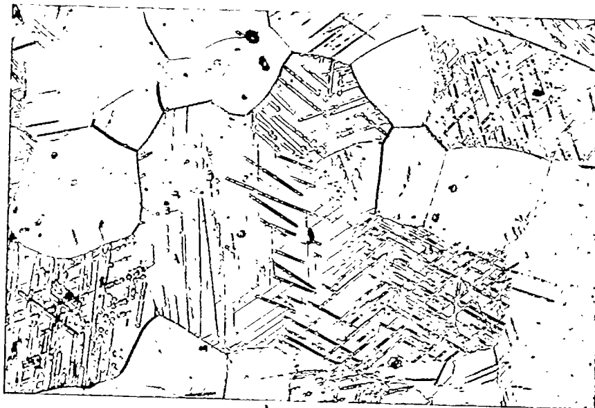
Figure 21.- Alloy 254 containing 70 percent cobalt and 30 percent chromium. Electrolytically polished and etched with reagent 1; quenched from beta phase field at 900° C to room temperature; Widmanstätten precipitate is probably a sigma-phase precipitate formed on cooling; X400.
