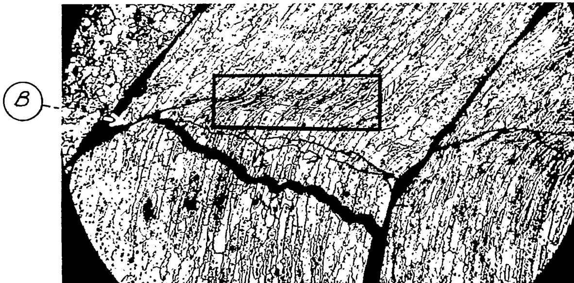
Figure 16.- Cracks at A in figure 15. Crack started at B, began to move through heavily cold-worked area (rectangular box), and changed direction probably because of higher stressing along line of eventual failure. X100.
