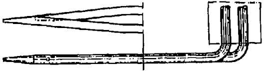
Fig. 9 Pitot-static nozzle of M.H. Darcy and M.E. Basin, 1865
