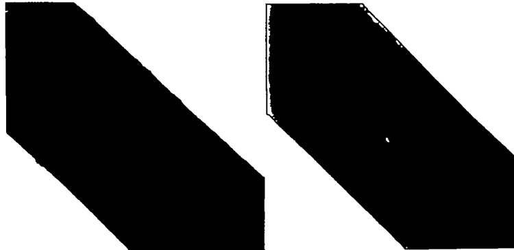
(b) Sample B; etched tungsten; nominal diameter, 0.0002 inch; actual diameter, 0.000199 inch; X5450.
