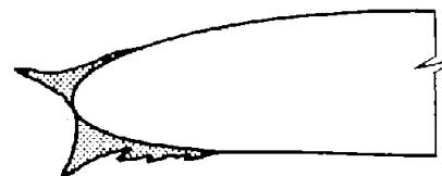
(c) Double-peak mushroom-type glaze ice. Datum air temperature, 25^{\circ} to 30^{\circ} F; moderate to high rate of water catch.
