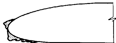
(b) Glaze ice. Datum air temperature, 25^{\circ} F; low rate of water catch.
