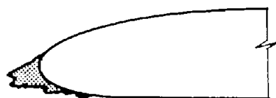
(a) Rime ice. Datum air temperature, 0^{\circ} F.
