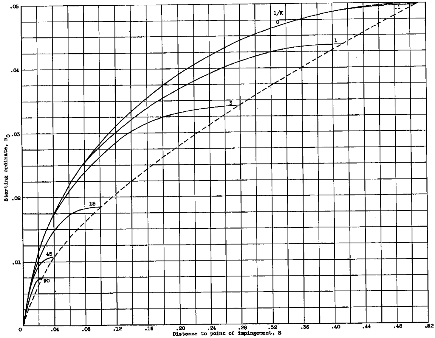
Figure 4. - Starting ordinate as function of distance along surface to point of impingement.
