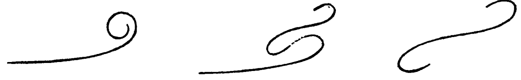
Shape of rolling-up vortex sheet
