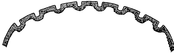
(a) Approximate tread shape of tires A and B at beginning of test.
